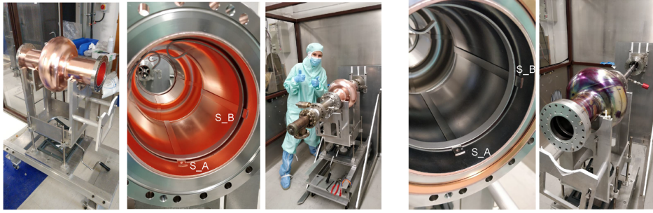
Figure 4.15.: First Nb thin-film-coated 802 MHz cavity at CERN. The three leftmost figures show the copper cavity before coating including the clean-room assembly. The two rightmost figures show the cavity after the Nb coating [226].
