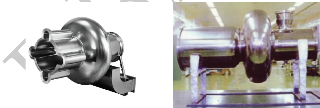
Figure 4.8.: The 500 MHz CESR cavity (left) [199], and 508 MHz KEKB cavity (right) [200]
