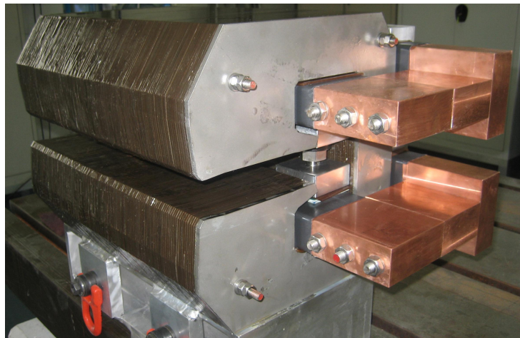
Figure 8.8: One of the 400 mm long model magnets made at CERN with interleaved laminations.
