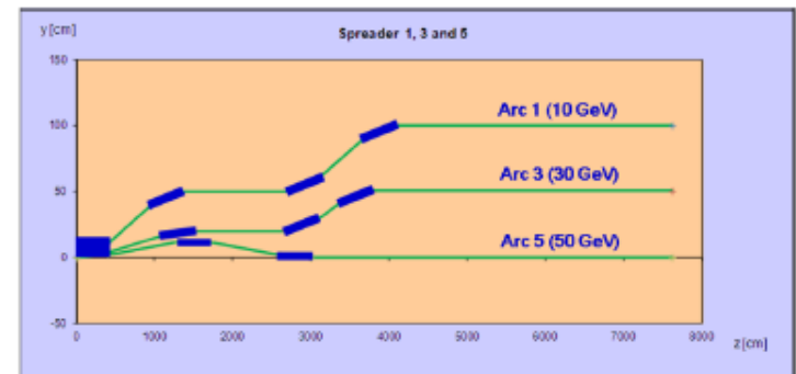
1→3 beam spreader design
