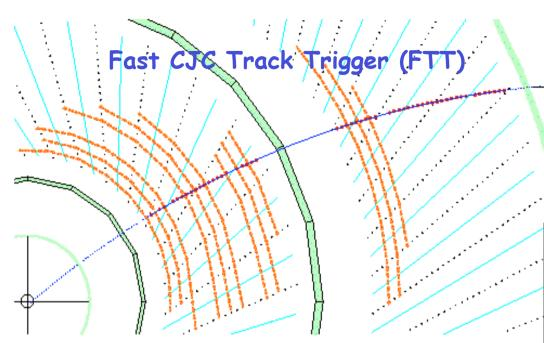
Level 1 reconstruction of hits (Qt) and r-phi-tracks in ~30 FEM boards with 5 APEX chips and 30 FADCs (10bit)
