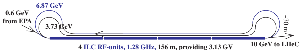
Figure 7.67: Recirculator using 4 ILC modules.
