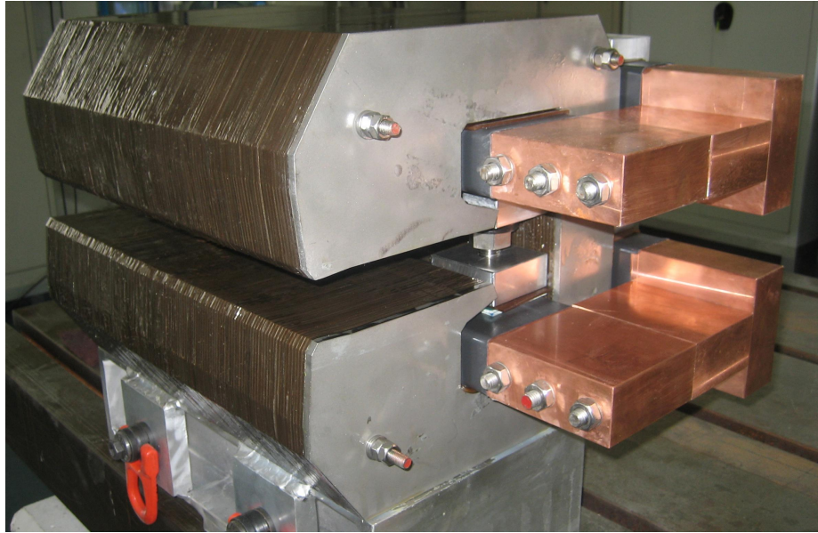
Figure 9.8: One of the 400 mm long model magnets made at CERN with interleaved laminations.
