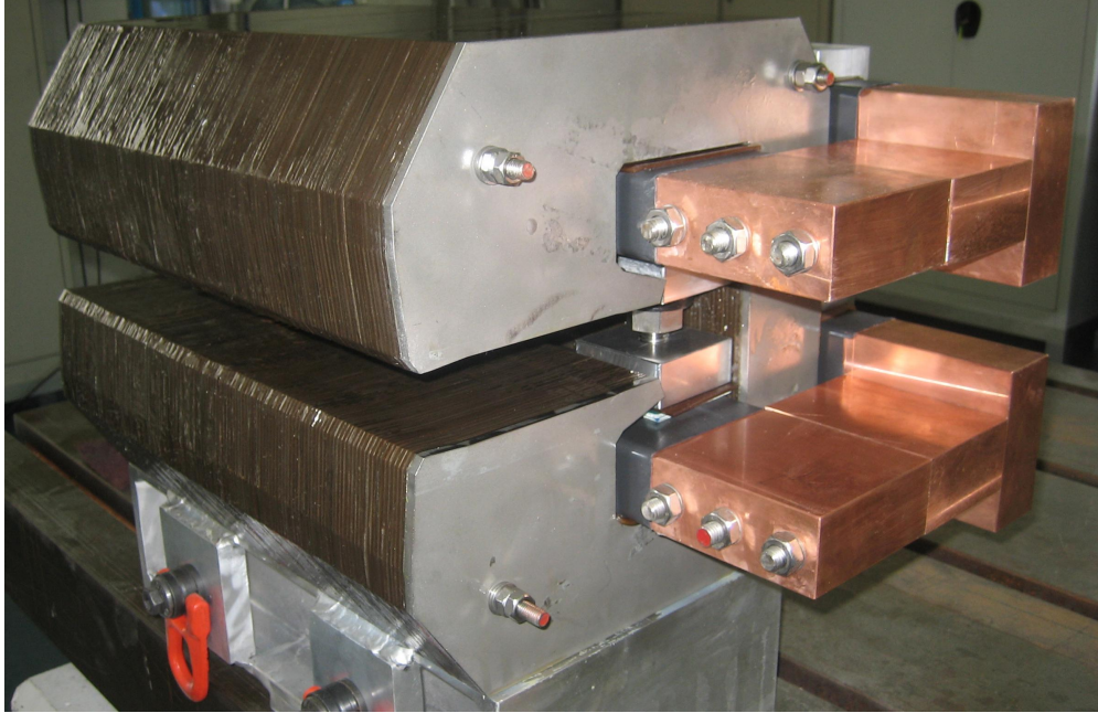
Figure 9.10: 400 mm long RR dipole model with interleaved laminations
