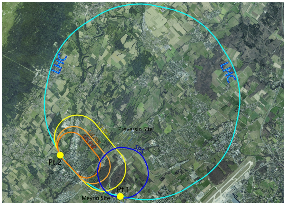
Figure 8.46: Racetrack options proposed for LHeC at Point 2 LHC. The color coding illustrated different options with 1/3 , 1/4 and 1/5 of the LHC circumference, resulting in different electron beam energies.
