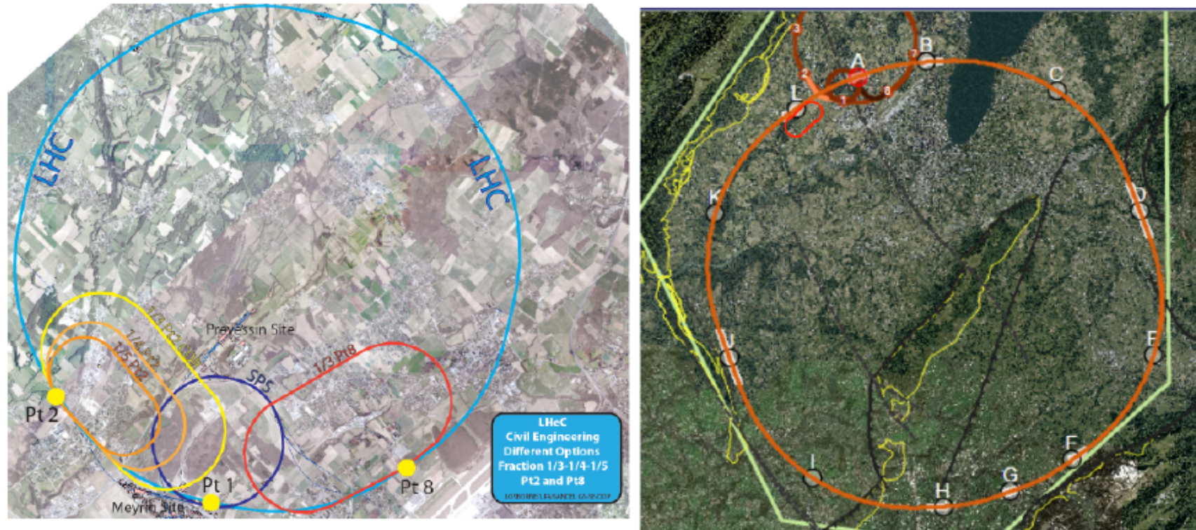
Figure 2: Possible locations of the ERL racetrack electron accelerator for the LHeC (left) and the FCC-he (right). The LHeC is shown to be tangential to Point 2 and Point 8. For Point 2 three sizes are drawn corresponding to a fraction of the LHC circumference of 1/3 (outer, default with E_e = 60 GeV), 1/4 (the size of the SPS, E_e = 56 GeV) and 1/5 (most inner track, E_e = 52 GeV). To the right one sees that the 8.9 km default racetrack configuration appears to be rather small as compared to the 100 km ring of the FCC. Present considerations suggest that Point L may be preferred as the position of the ERL, while two GPDs would be located at A and G.
