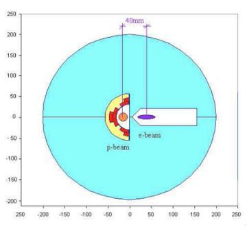
First p beam lens: septum quadrupole. Cross section and Field calculation
