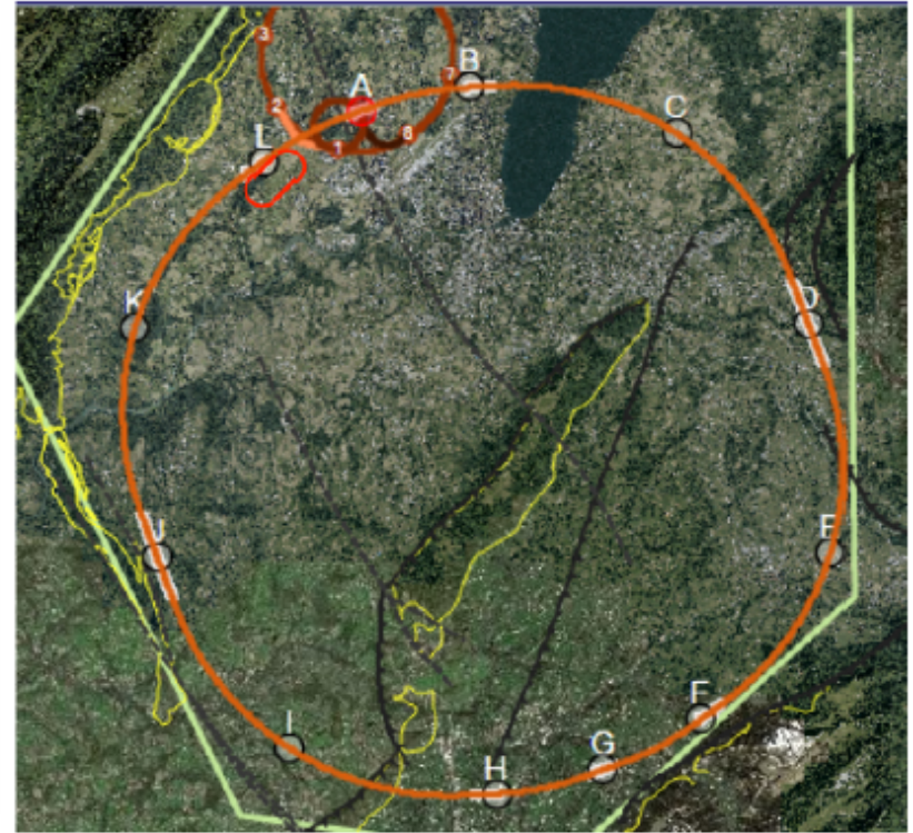
Figure 2: Possible locations of the ERL racetrack electron accelerator for the LHeC (left) and the FCC-he (right). The LHeC is shown to be tangential to Point 2 and Point 8. For Point 2 three sizes are drawn corresponding to a fraction of the LHC circumference of 1/3 (outer, default with E_e = 60 GeV), 1/4 (the size of the SPS, E_e = 56 GeV) and 1/5 (most inner track, E_e = 52 GeV). To the right one sees that the 8.9 km default racetrack configuration appears to be rather small as compared to the 100 km ring of the FCC. Present considerations suggest that Point L may be preferred as the position of the ERL, while two GPDs would be located at A and G.
