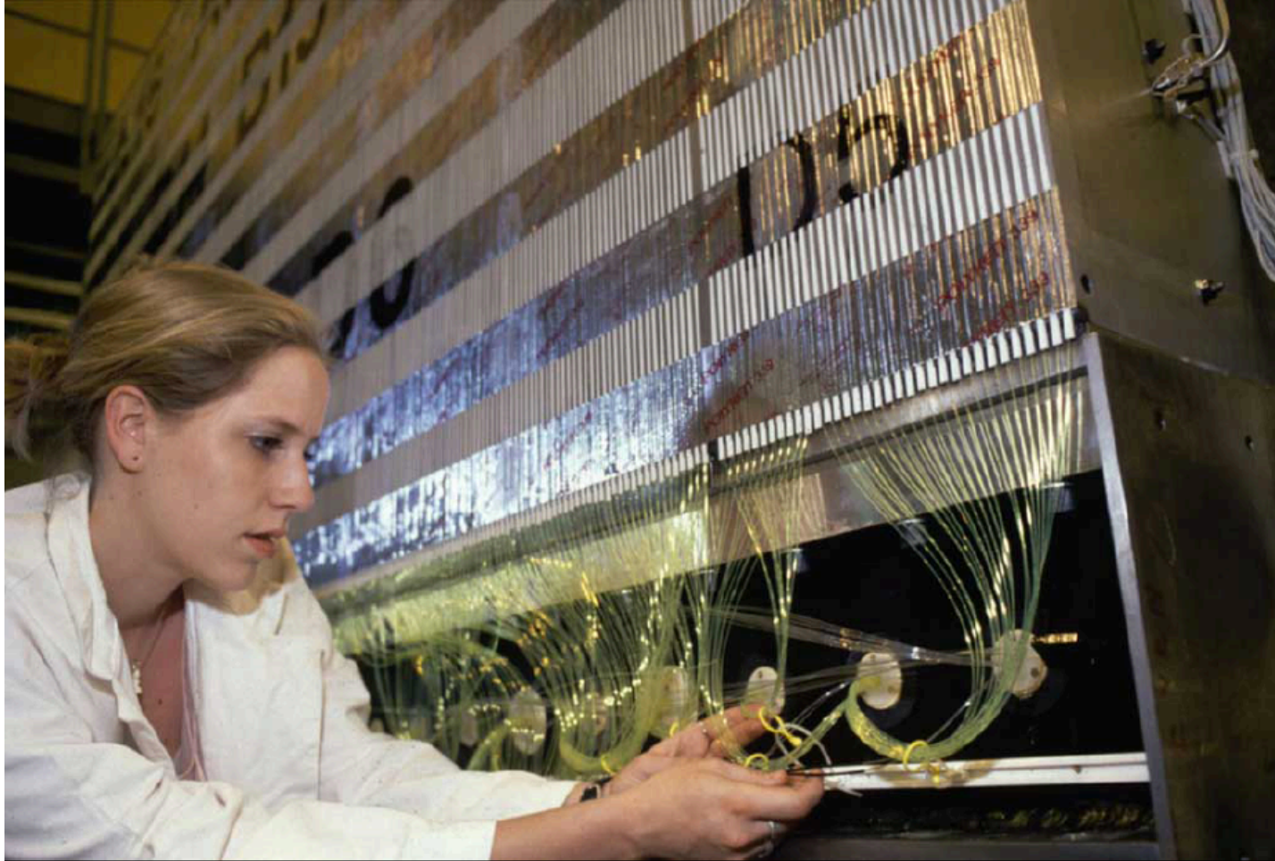
Scintillator and Fe absorber, read out perpendicular to beam axis
