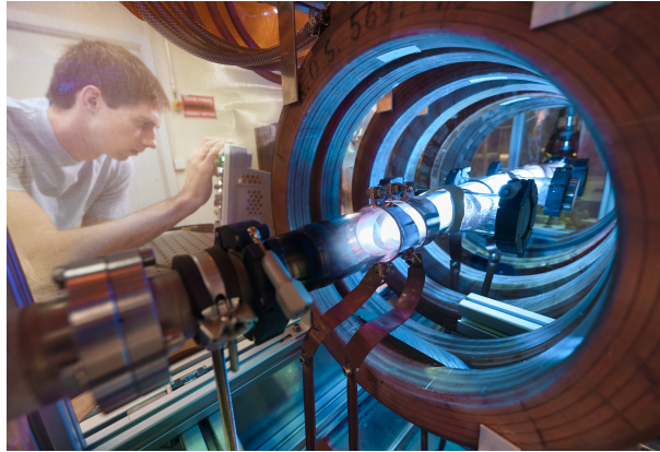
Fig. 4.10: 1 m prototype of a scalable Helicon plasma source. Image credit: CERN
