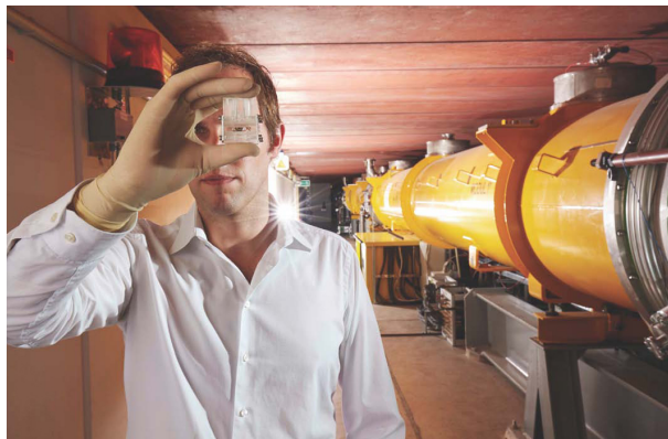
Fig. 4.2: A plasma cell is shown here in comparison to the super-conducting accelerator FLASH at DESY. Image credit: DESY, H. Mueller-Elsner
