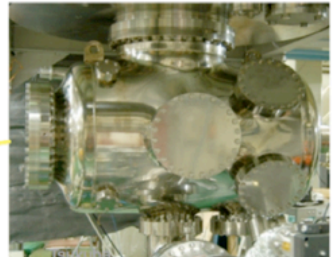
gun chamber made of titanium
