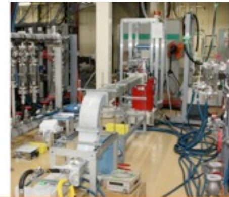
30kW CW Klystron for injector SCC
