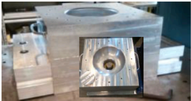
Fixture for female die with blank holder
