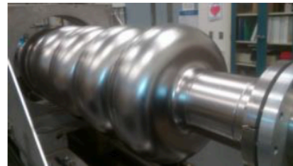
Five-cell cavity on tuning bench
