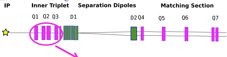
Implementation of new triplet Q1-Q3 with aperture for 2 proton beams and one electron beam → current studies based on layout WITHOUT Crab Cavities!
