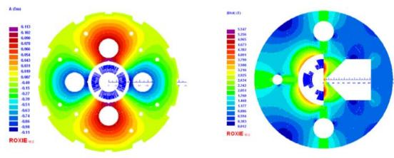
Consideration of the magnets for the LHeC included the design of a half quadrupole for Q1 given the short distance between the proton beam and the electron beam
