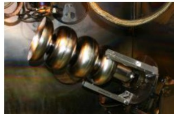
Five-cell cavity in EBW machine prepared for subsequent dumbbell and endgroup welding with both outside and inside welds in tilted position
