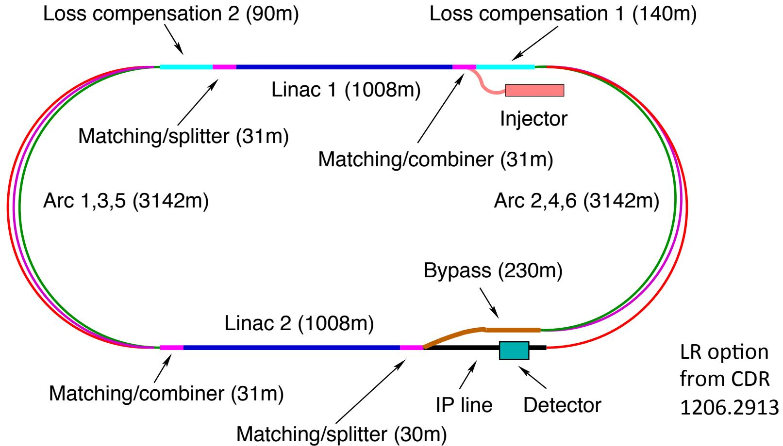
**60 GeV electron beam energy,  $L = 10^{33} \text{ cm}^{-2}\text{s}^{-1}$ ,  $\sqrt{s} = 1.3 \text{ TeV}$ :  $Q^2_{\max} = 10^6 \text{ GeV}^2$ ,  $10^{-6} < x < 1$**
