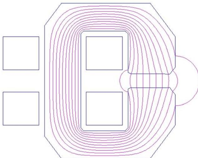
Figure 10.8: Bending magnets for the LR recirculator
