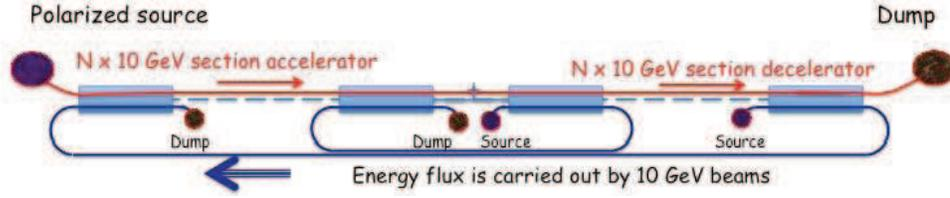
Figure 9.9: Highest-energy high-luminosity ERL option based on two straight linacs and multiple 10-GeV energy-transfer beams [?].
