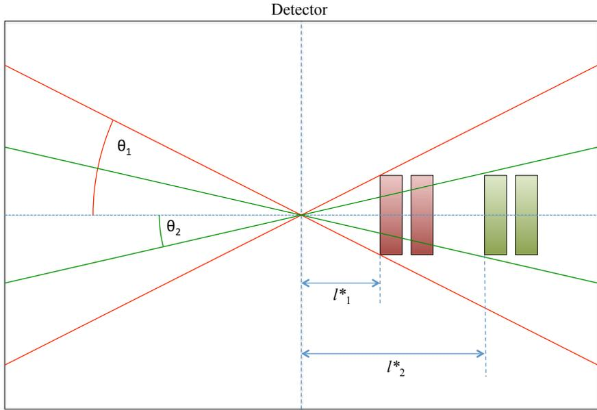
Figure 8.22: Graphical representation of acceptance.  $\theta_1$  shows a lower acceptance cone, while  $\theta_2$  shows a higher acceptance cone. For machine elements of constant diameter, higher acceptance increases  $l^*$ .
