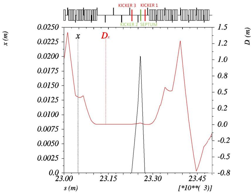
Figure 10.26: A closed orbit bump of 20 mm is generated by three kickers installed in the dispersion free region located at the right side of the bypass around ATLAS (electron beam moves from right to left in the Figure).
