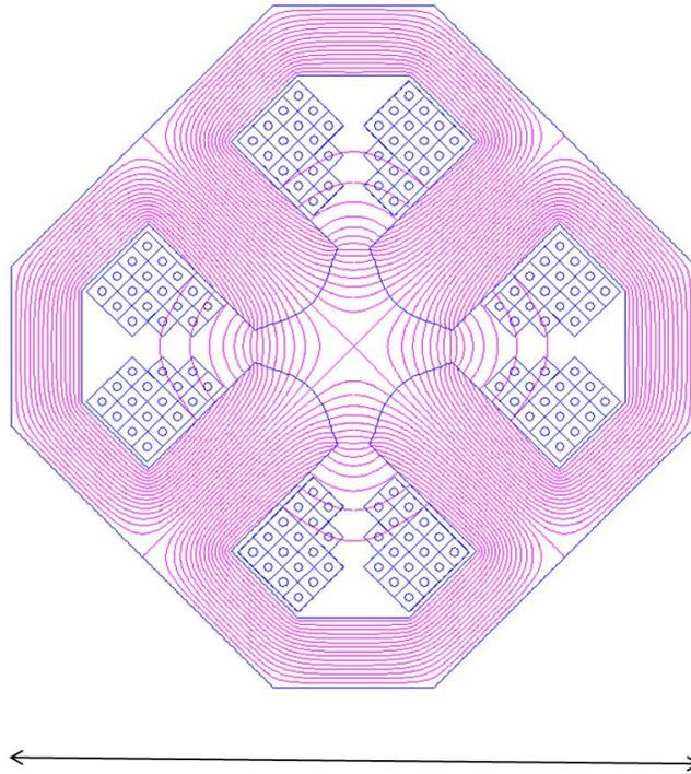
Figure 10.12: Insertion and by-pass quadrupole magnets for the RR Option
