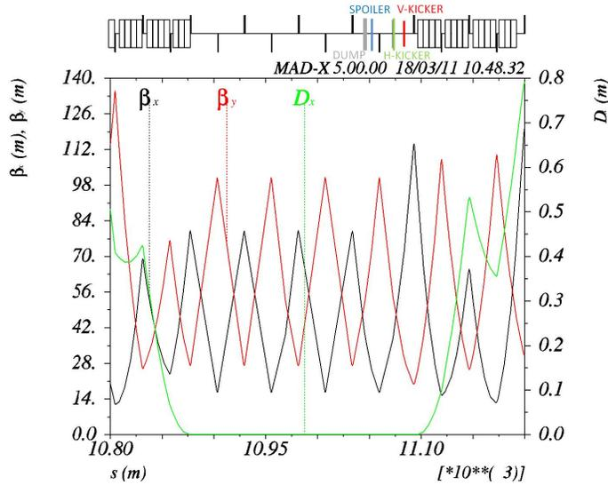
Figure 10.28: The optics in the region of the CMS bypass where the beam dump system could be installed is shown. The system consists of two kickers, one spoiler and a Carbon-composite absorber which are installed in the dispersion free region of the bypass at the right side of CMS (beam proceeds from right to left in the Figure).
