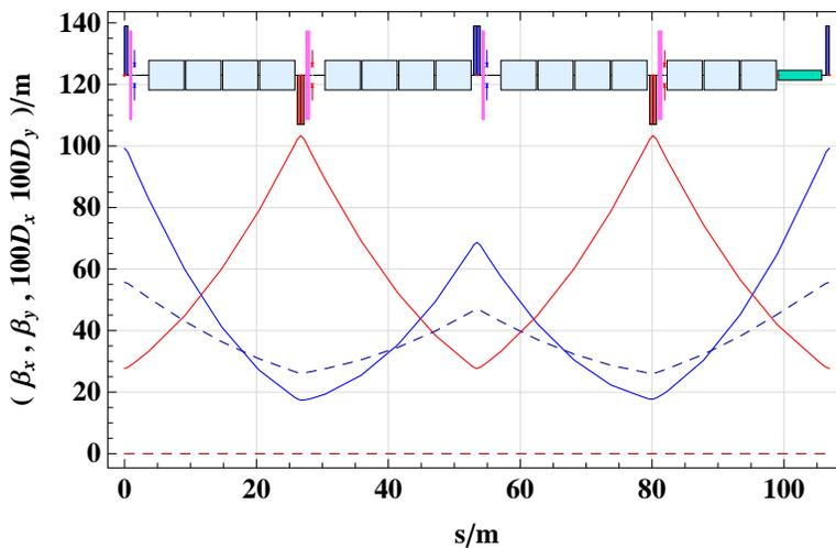
Figure 8.3: Electron ring arc cell optics.
