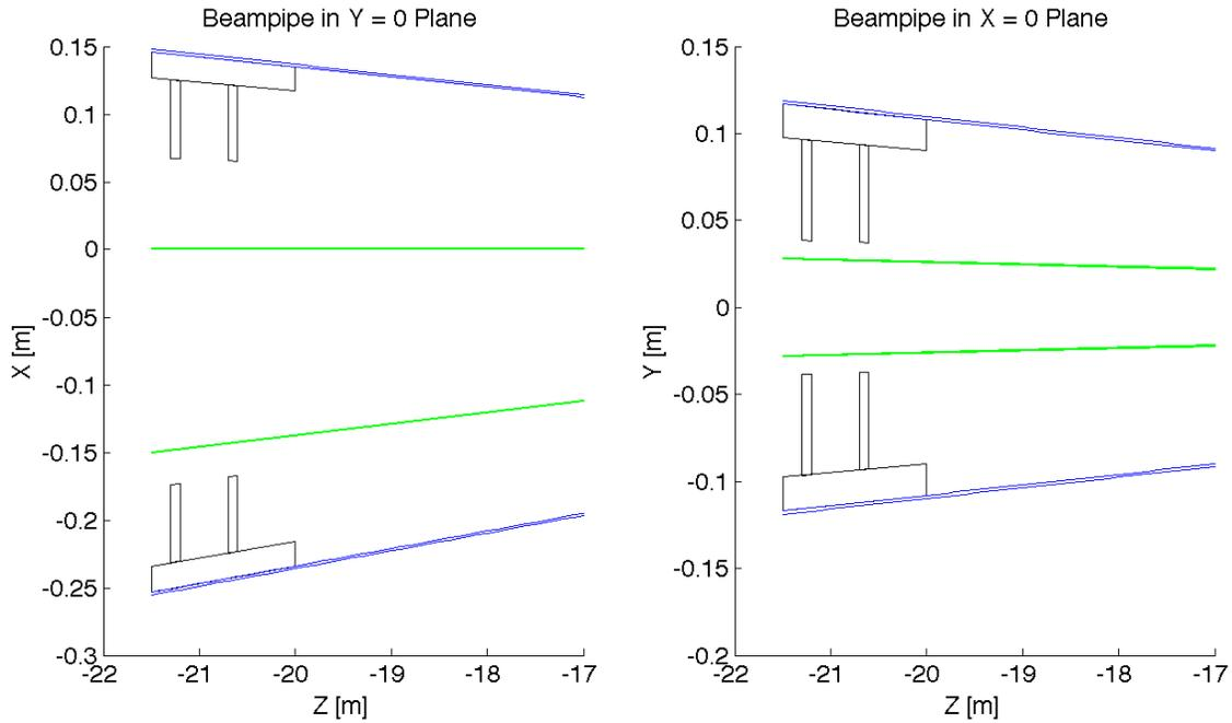
Figure 8.44: High Acceptance: Beampipe Cross Sections
