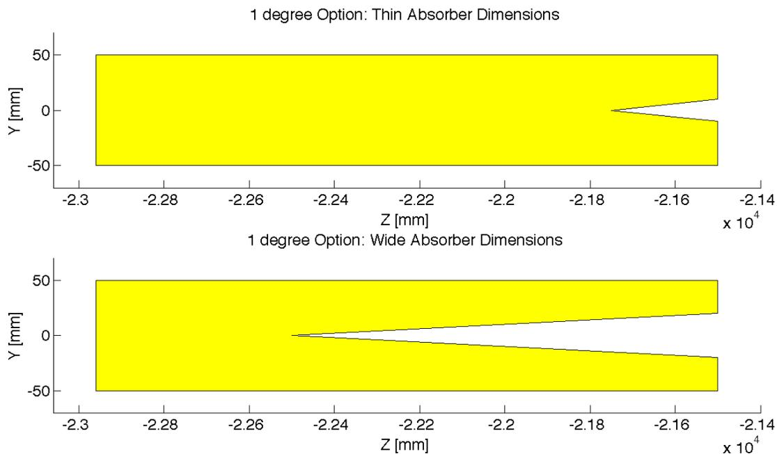
Figure 8.43: 1 deg: Absorber Dimensions
