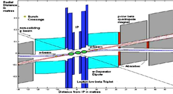
Figure 8.19: LHeC interaction region including the location of the first parasitic bunch encounters where due to the crossing angle of 1 mrad a sufficient beam separation is achieved.
