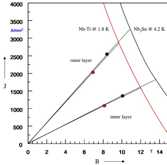
Figure 10.5: Working points on the load-line for both Nb-Ti and Nb<sub>3</sub>Sn variants of the half quadrupole for Q1.
