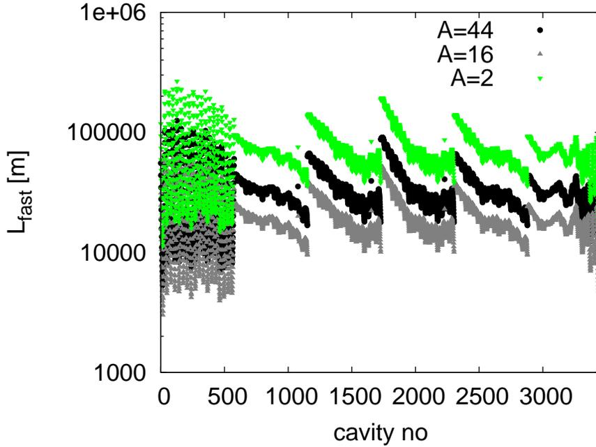
Figure 9.39: The instability length of the beam-ion instability assuming a very conservative partial pressure of  $10^{-11}$ hPa for each gas.
