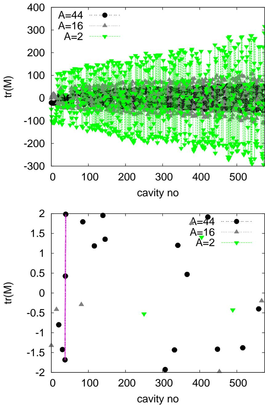
Figure 9.38: The trace of the transfer matrix for  $H_2^+$ ,  $CH_4^+$  and  $CO_2^+$  ions in presence of a clearing gap. Values above 2 or below  $-2$  indicate that the ions will not be trapped.
