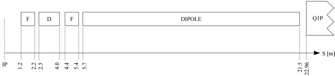
Figure 8.23: Layout of machine elements in the High Luminosity IR. Note that the left side of the IR is symmetric.
