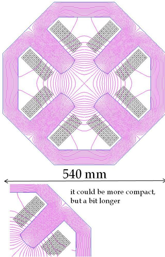
Figure 10.13: Quadrupoles for the 10 GeV linacs of the LR option
