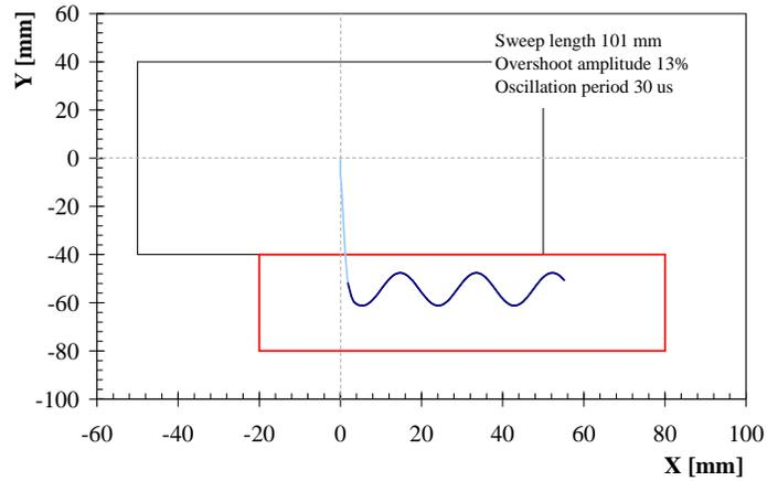
Figure 10.29: A vertical and a horizontal kicker are used to dilute the beam on the dump absorbing block.
