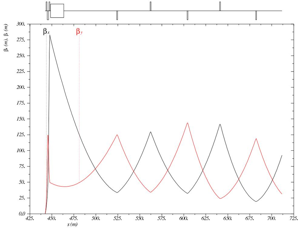
Figure 8.26:  $\beta$  functions in both planes for the High Luminosity IR layout, from the IP to the start of the right dispersion suppressor. Note that  $s$  is relative to the ring, which begins at the left side of the left dispersion suppressor of IP2.
