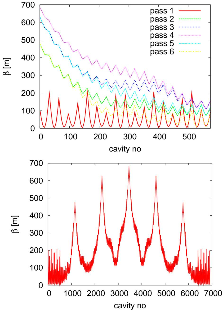
Figure 9.31: Beta-functions in the first linac. On the top, the beta-functions of the six different beam passages in the first linac are shown. On the bottom, the beta-function as seen by the beam during his stay in the linacs are shown.
