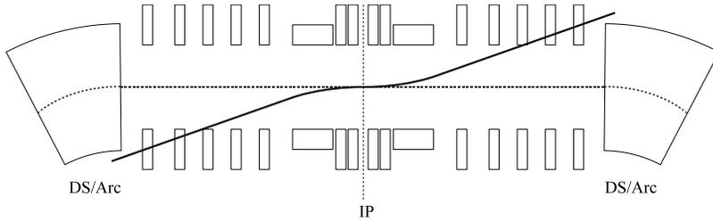
Figure 8.27: Graphical representation of misaligned LSS/IR geometry. With beam steering in the IR and no compensation in the LSS, the electron beam no longer lines up with the ring lattice reference orbit. Diagram is not to scale and does not represent the correct optical layout of the IR nor the LSS.
