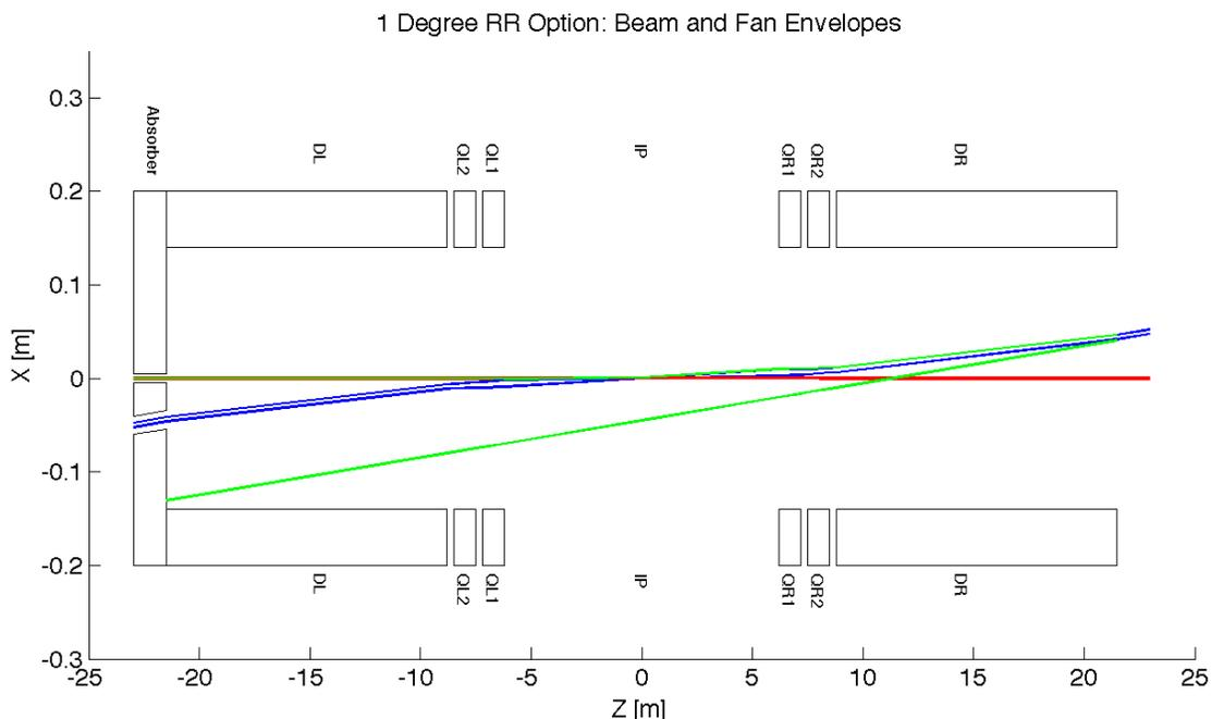
Figure 8.40: High Acceptance: Beam Envelopes in Z
