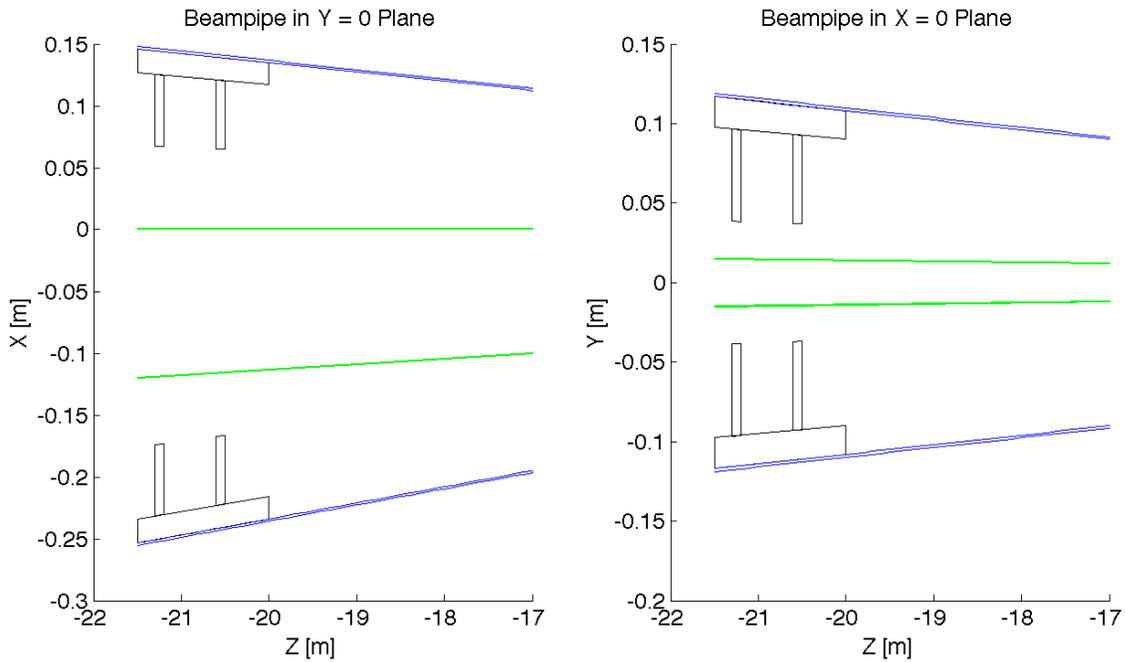
Figure 8.38: High Luminosity: Beampipe Cross Sections
