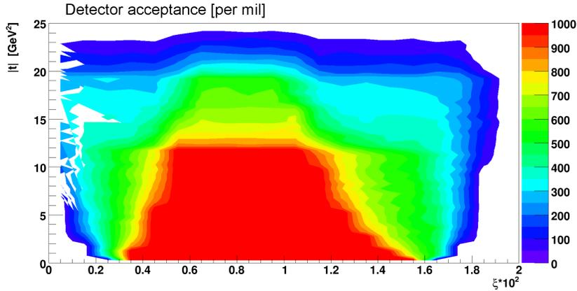
Figure 13.2: The acceptance for a proton detector placed at 420m from the interaction point is shown as function of the momentum loss  $\xi$  and the fourmomentum-transfer squared  $t$ . The color legend runs from 0‰(no acceptance) to 1000‰(full acceptance).
