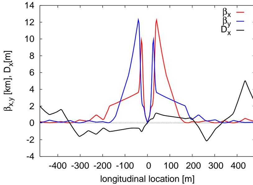
Figure 9.15: Optics functions for main proton beam.
