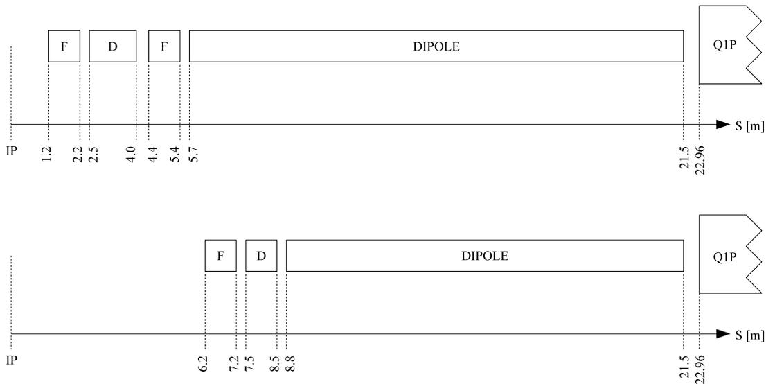
Figure 8.32: Scale comparison of the layouts for the High Luminosity and High Acceptance designs. Note the large difference in  $l^*$ .
