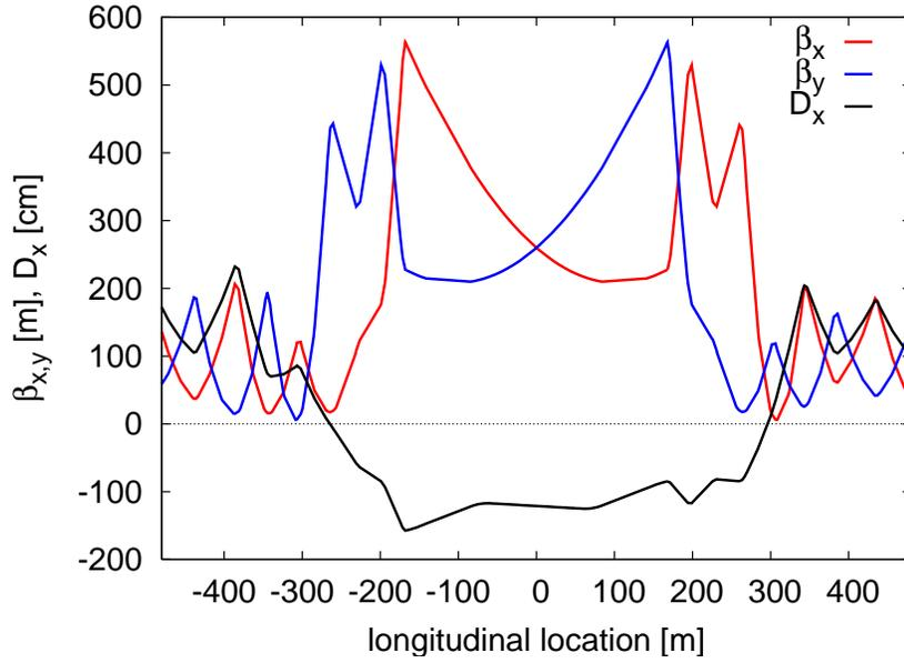
Figure 9.17: Optics functions for the non-colliding proton beam without triplets.
