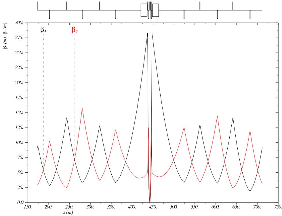
Figure 8.25:  $\beta$  functions in both planes for the High Luminosity IR layout, from the end of the left dispersion suppressor to the start of the right dispersion suppressor. Note that  $s$  is relative to the ring, which begins at the left side of the left dispersion suppressor of IP2.
