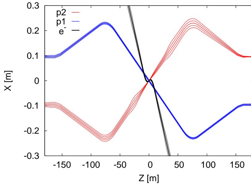
Figure 9.13: LHeC interaction region displaying the two proton beams and the electron beam trajectories with  $5\sigma$  and  $10\sigma$  envelopes.
