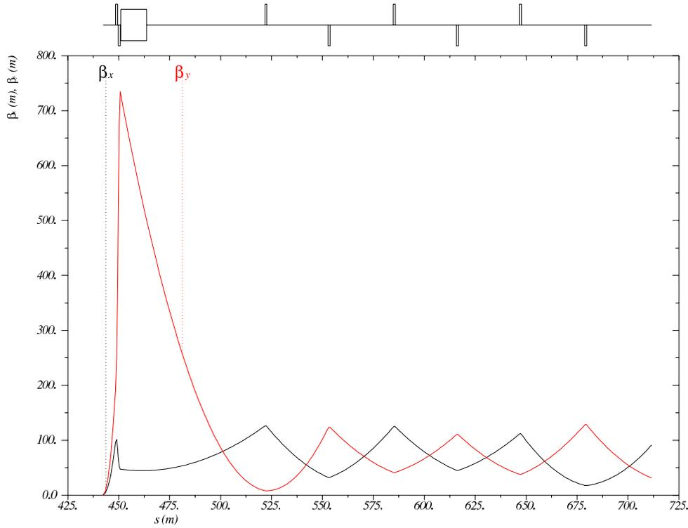
Figure 8.31:  $\beta$  functions in both planes for the High Luminosity IR layout, from the IP to the start of the right dispersion suppressor. Note that  $s$  is relative to the ring, which begins at the left side of the left dispersion suppressor of IP2.
