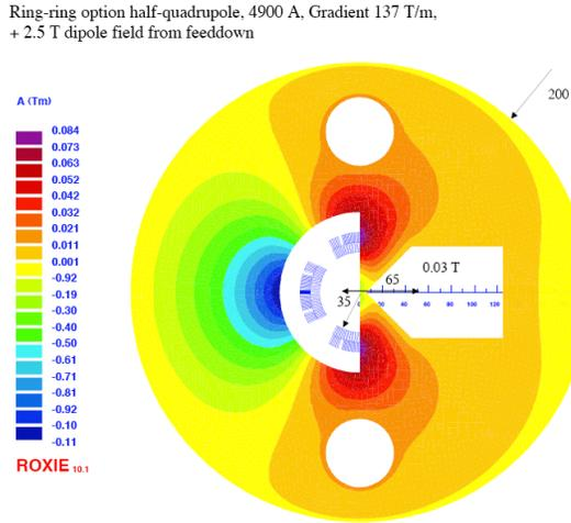
Figure 8.18: Super conducting half quadrupole in the proton lattice: The electron beam will pass on the right and side of the mirror plate in a quasi field free region.
