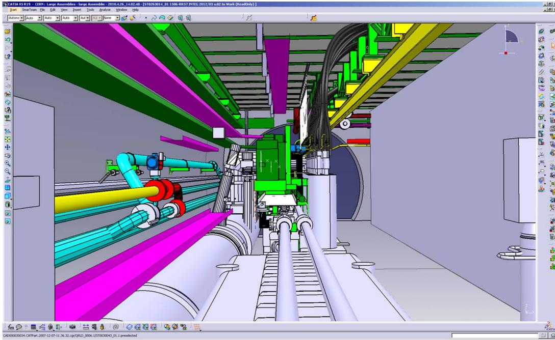
Figure 8.57: A typical big current feedbox (DFBA)
