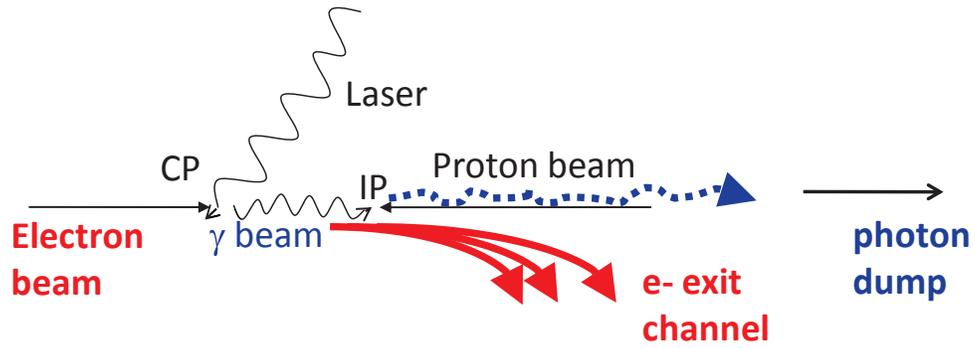
Figure 9.10: Schematic of  $\gamma$ - $p/A$  collision; prior to the photon-hadron interaction point (IP), the electron beam is scattered off a several-J laser pulse at the conversion point (CP).
