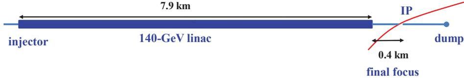
Figure 9.8: Pulsed single straight 140-GeV linac for highest energy ep collisions.
