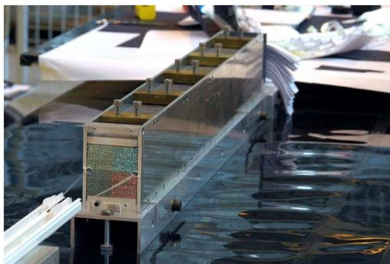
Figure 13.1: Photo of the Zero Degree Neutron Calorimeter (ZN) of ALICE experiment.
