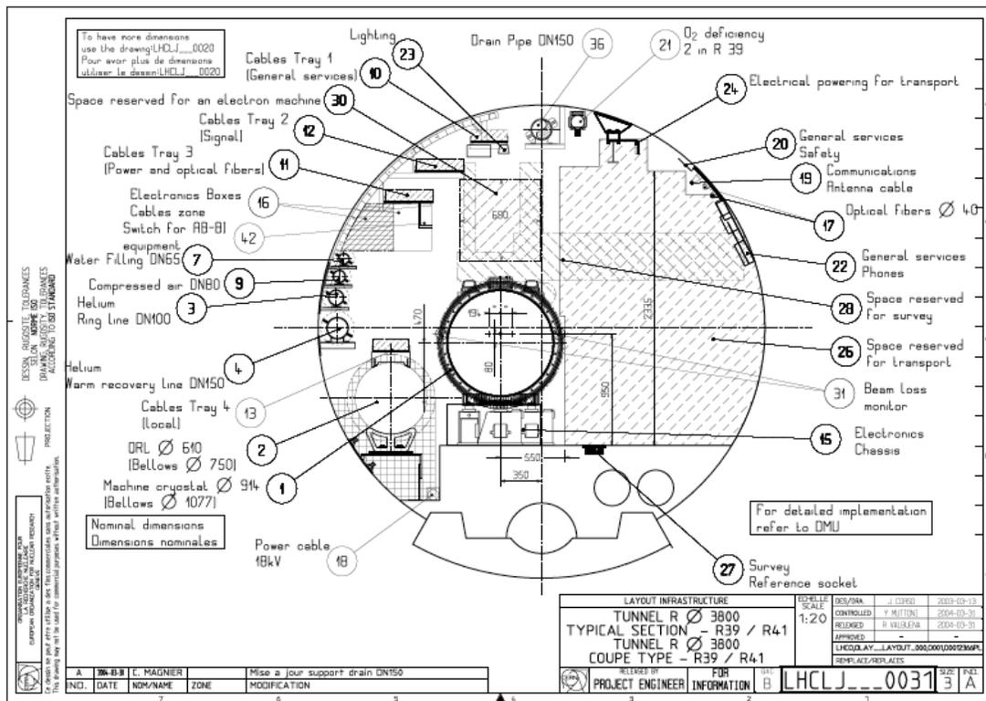
Figure 8.48: Cross-section of the LHC tunnel [?]
