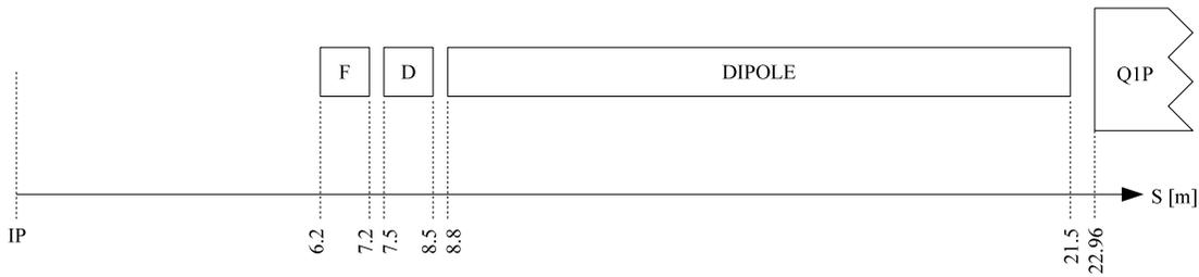
Figure 8.28: Layout of machine elements in the High Acceptance IR. Note that the left side of the IR is symmetric.
