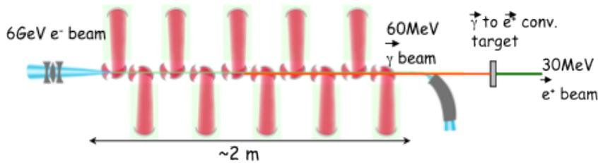
Figure 10.19: Layout based on Compton Linac for polarised  $e^+$ .
