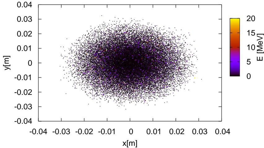
Figure 9.20: Distribution of the spent electron beam at 10 m from the IP. The Gaussian and rms sigmas are shown on the plot.
