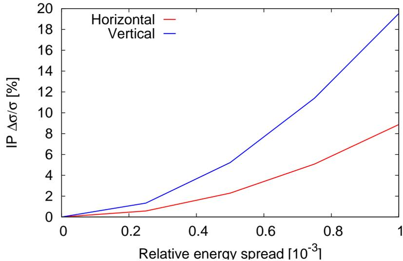
Figure 9.19: IP electron beam size versus relative energy spread of the beam.
