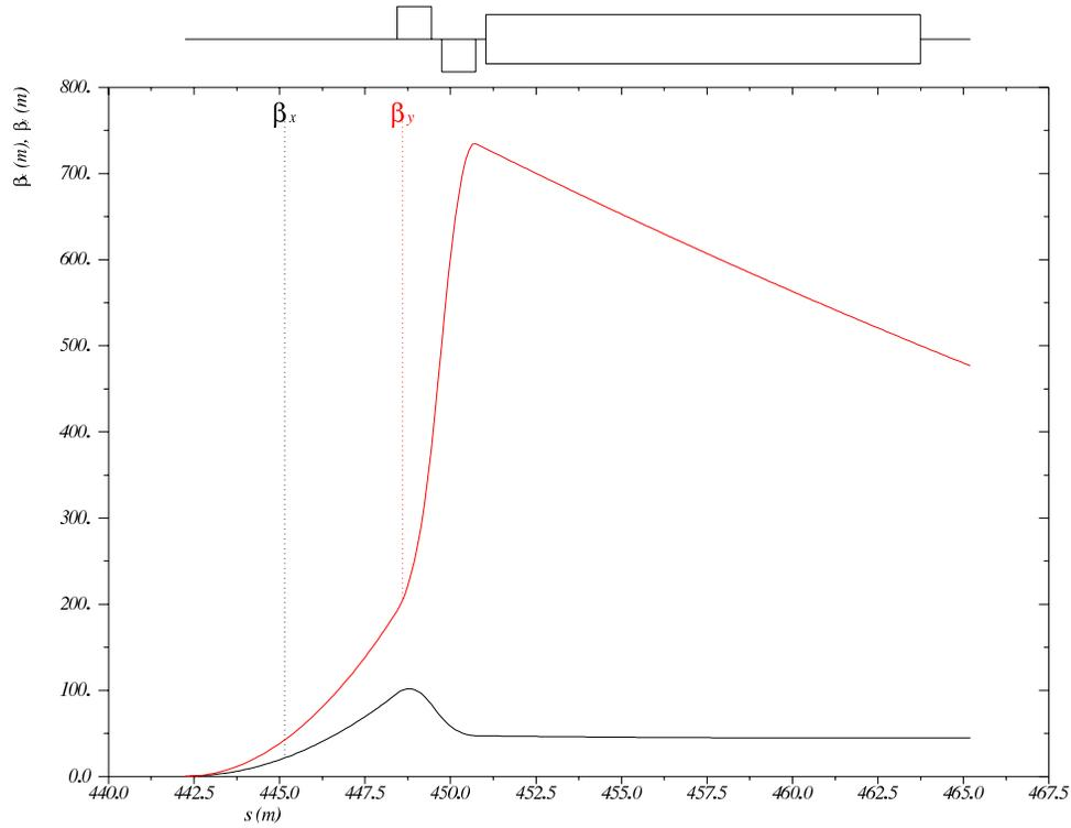
Figure 8.29:  $\beta$  functions in both planes for the High Acceptance IR layout, from the IP to the face of the final proton quadrupole at  $s = 23$  m. Note that  $s$  is relative to the ring, which begins at the left side of the left dispersion suppressor of IP2.
