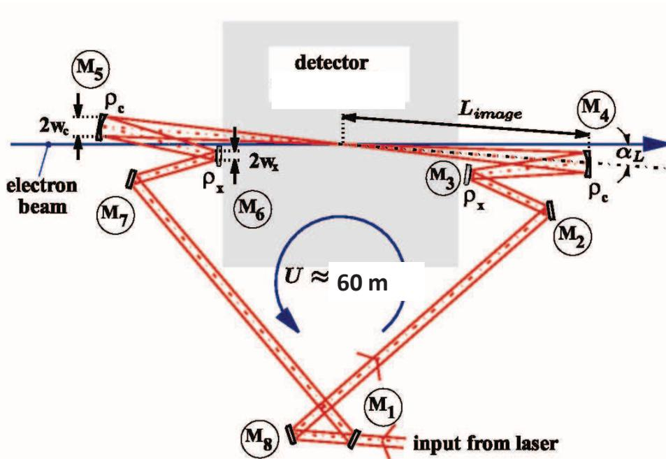
Figure 9.12: Recirculating mirror arrangement providing a laser-pulse path length of 60 m for pulse stacking synchronously with the arriving electron bunches (adapted from [?]).
