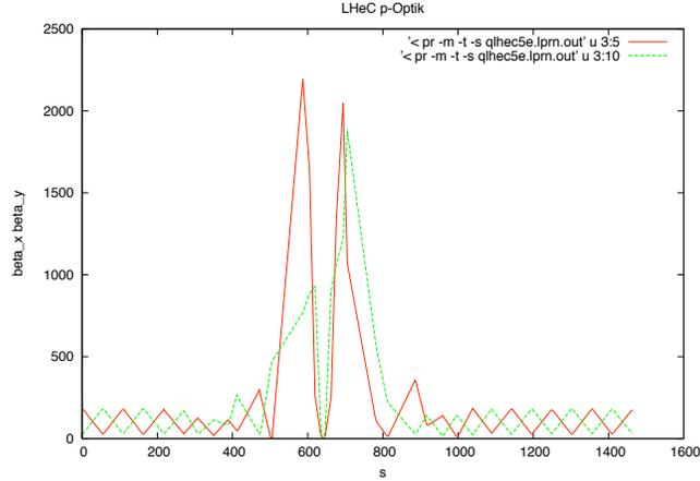
Figure 8.20: Proton optics for the LHeC interaction region. The gradients of the antisymmetric triplet lattice in the standard LHC have been modified to adopt for the requirements of the LHeC flat beam parameters.
