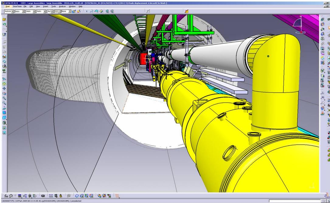
Figure 8.56: The cryogenic connection in point 3
