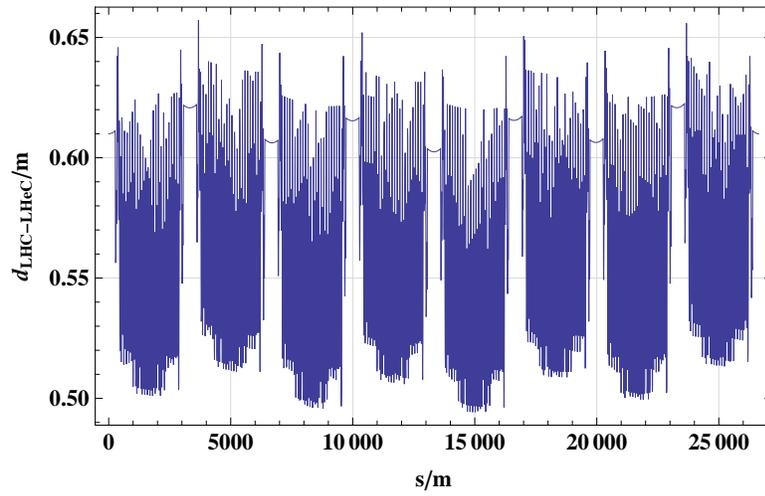
Figure 8.8: Distance between the idealized electron ring and the proton ring
