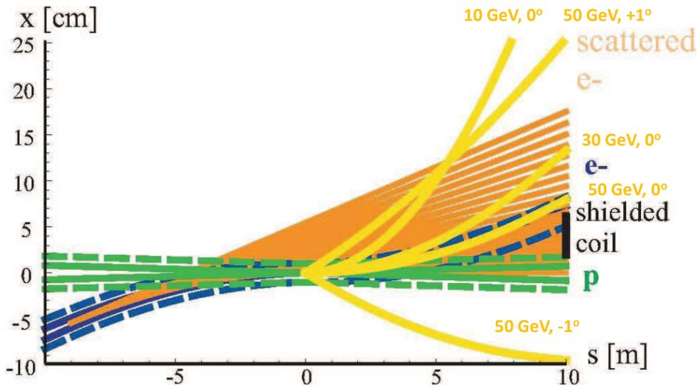
Figure 9.3: Example trajectories in the detector dipole fields for electrons of different energies and scattering angles, demonstrating an enhancement of the detector acceptance by the dipoles.
