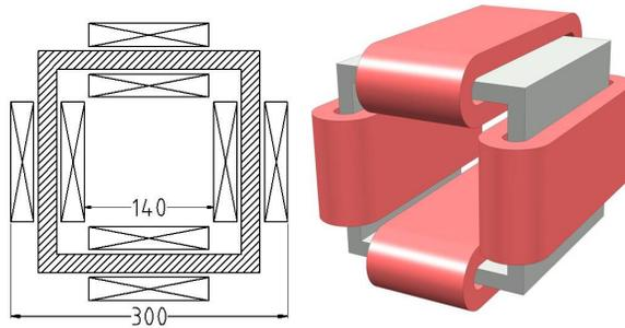
Figure 10.14: Combined function corrector magnets for the LR Option
