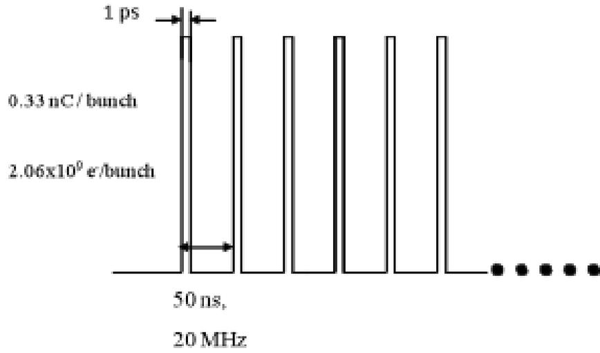
Figure 10.16: Beam pattern at IP
