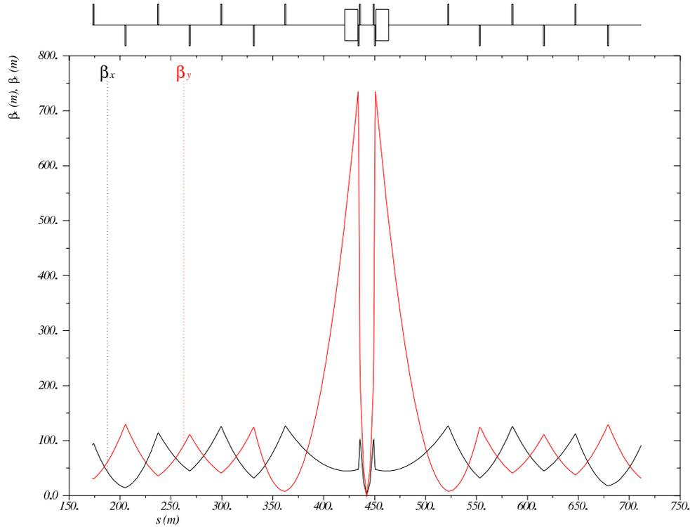
Figure 8.30:  $\beta$  functions in both planes for the High Acceptance IR layout, from the end of the left dispersion suppressor to the start of the right dispersion suppressor. Note that  $s$  is relative to the ring, which begins at the left side of the left dispersion suppressor of IP2.
