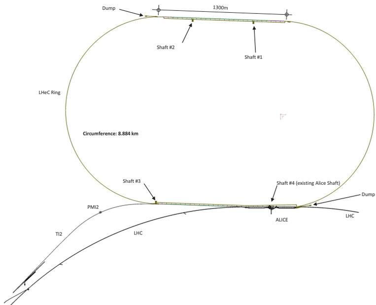
Figure 10.23: Two beam dumps are installed 90 m downstream the end of the long straight section of each linac for nominal operation and beam setup.
