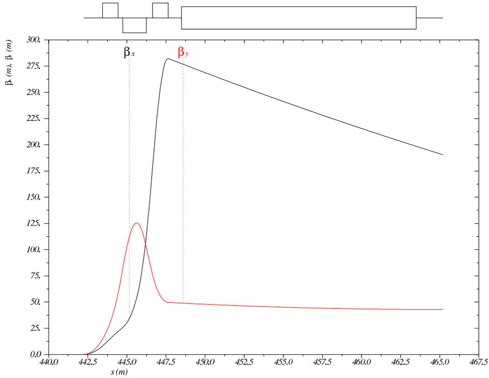
Figure 8.24:  $\beta$  functions in both planes for the High Luminosity IR layout, from the IP to the face of the final proton quadrupole at  $s = 23$  m. Note that  $s$  is relative to the ring, which begins at the left side of the left dispersion suppressor of IP2.
