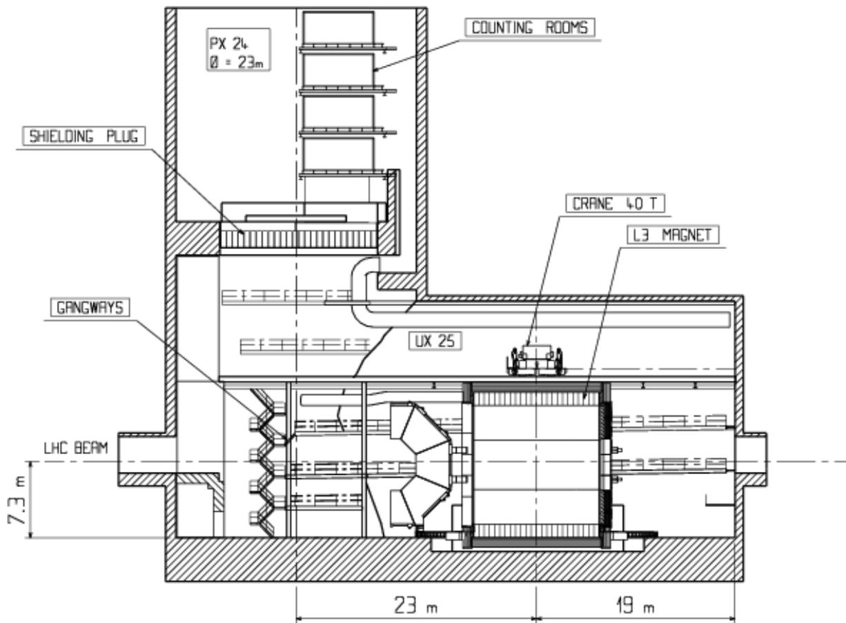
Figure 11.2: Cross section of the IP2 Caverne with the Alice detector inside the L3 magnet.
