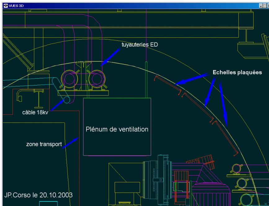
Figure 8.58: Air-duct in LSS7 [?]
