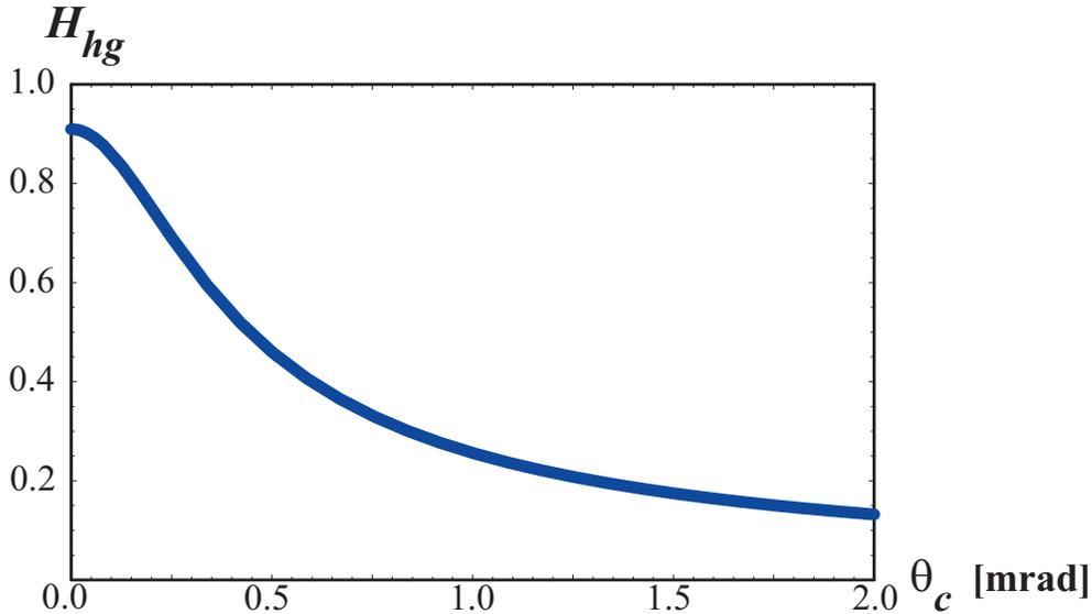
Figure 9.1: Geometric luminosity loss factor  $H_{hg}$ , (9.2), as a function of the total crossing angle
