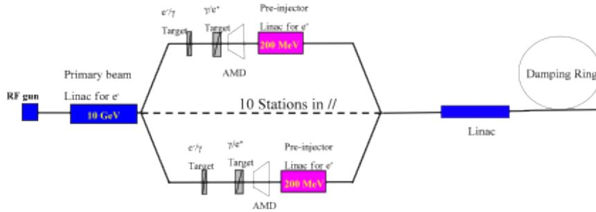
Figure 10.18: Possible layout with unpolarised  $e^+$  for the LHeC injector (p-140 GeV).
