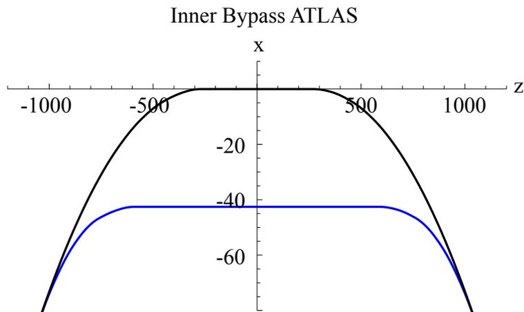
Figure 8.10: Inner Bypass around Point 1. The Bypass is shown in blue, The LHC proton ring in black.
