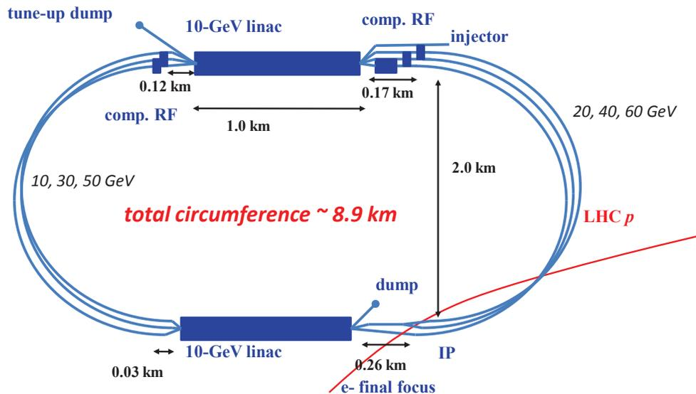
Figure 9.5: LHeC ERL layout including dimensions.
