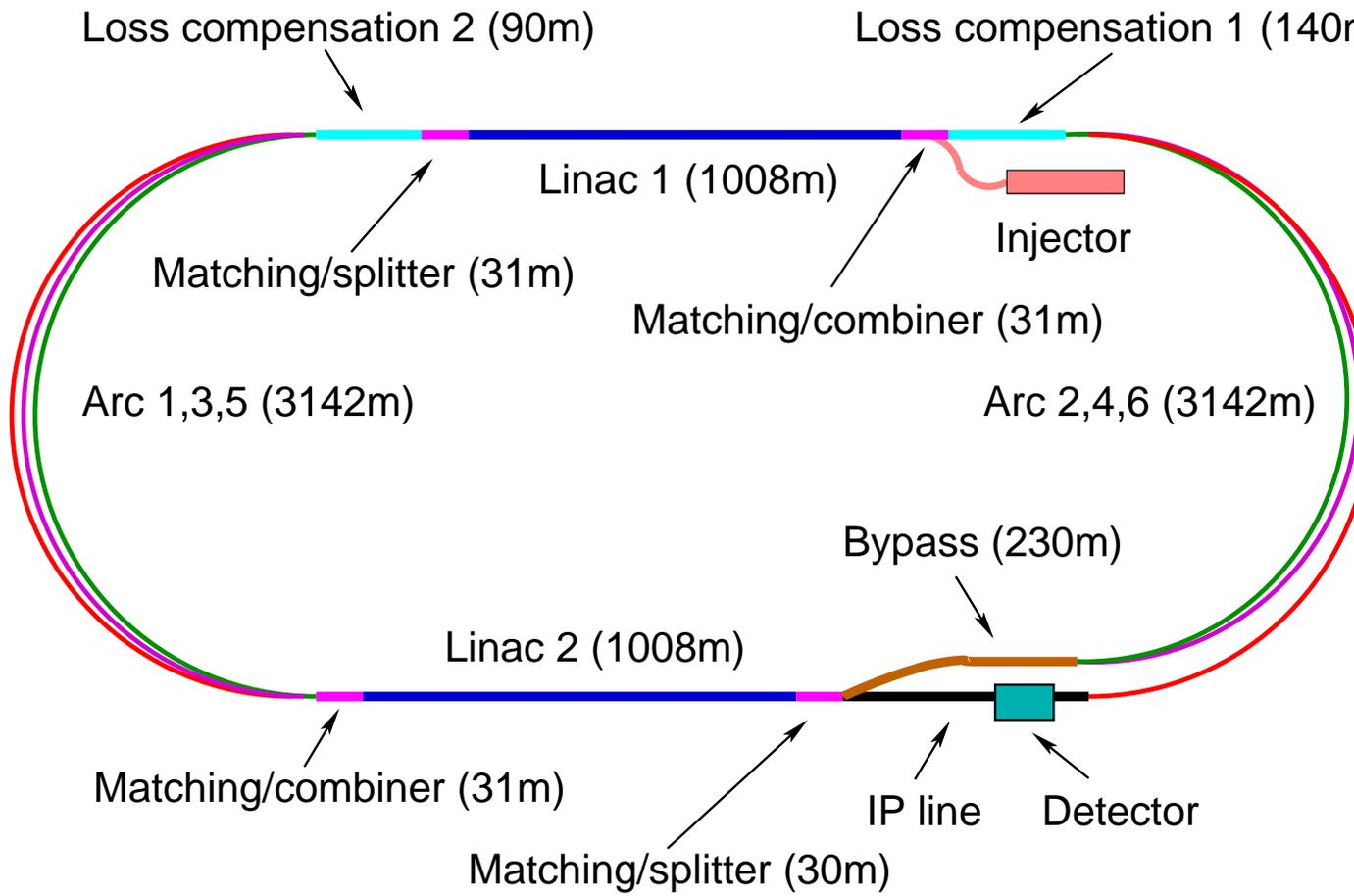
Figure 9.29: The schematic layout of the recirculating linear accelerator complex.
