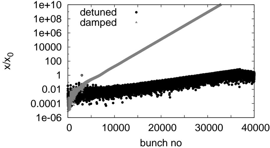
Figure 9.36: Multi-bunch beam break-up for the SPL cavities. In one case only damping, in the other case only cavity-to-cavity mode detuning is present.
