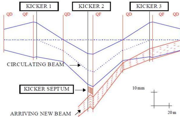
Figure 10.25: layout of mismatched injection system. To minimise kicker strengths the magnets are located near focusing quadrupoles.
