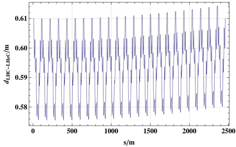
Figure 8.7: Horizontal distance between the proton and electron ring main arc.
