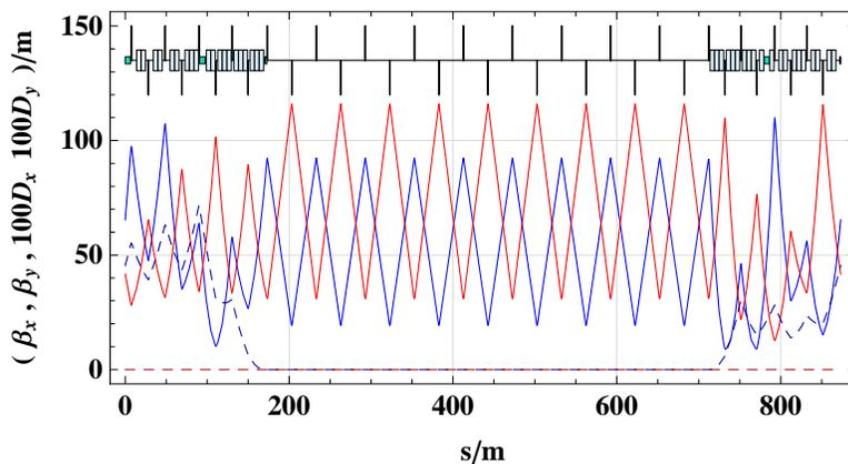
Figure 8.5: LHeC IR for even IRs, based on the DFBM configuration in point 2.
