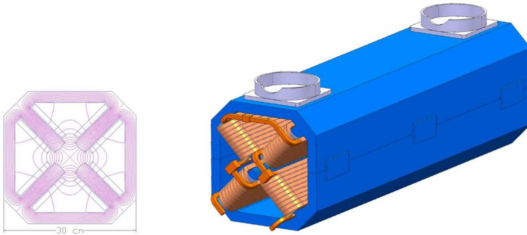
Figure 10.11: Arc quadrupole magnets for the RR Option
