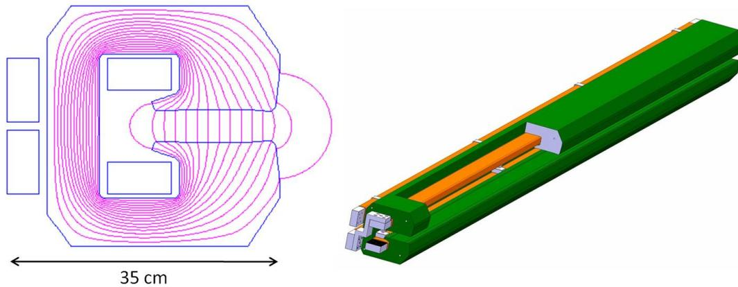
Figure 10.9: Bending magnets for the RR Option
