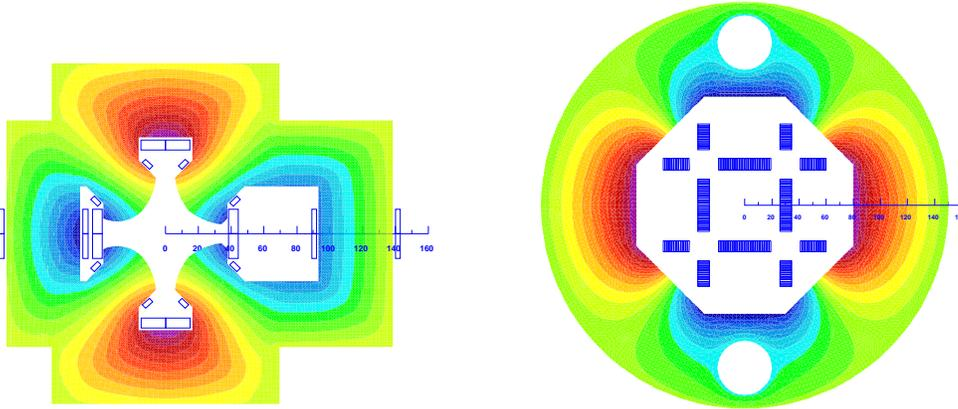
Figure 10.2: Cross-sections of insertion quadrupole magnets with iso-surfaces of the magnetic vector potential (field-lines). Left: Super-ferric, similar to the design presented in [?]. Right: Superconducting block-coil magnet as proposed in [?] for a coil-test facility.
