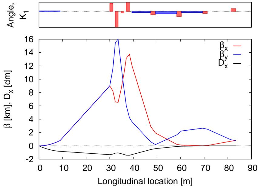
Figure 9.18: Optics of the electron beam.
