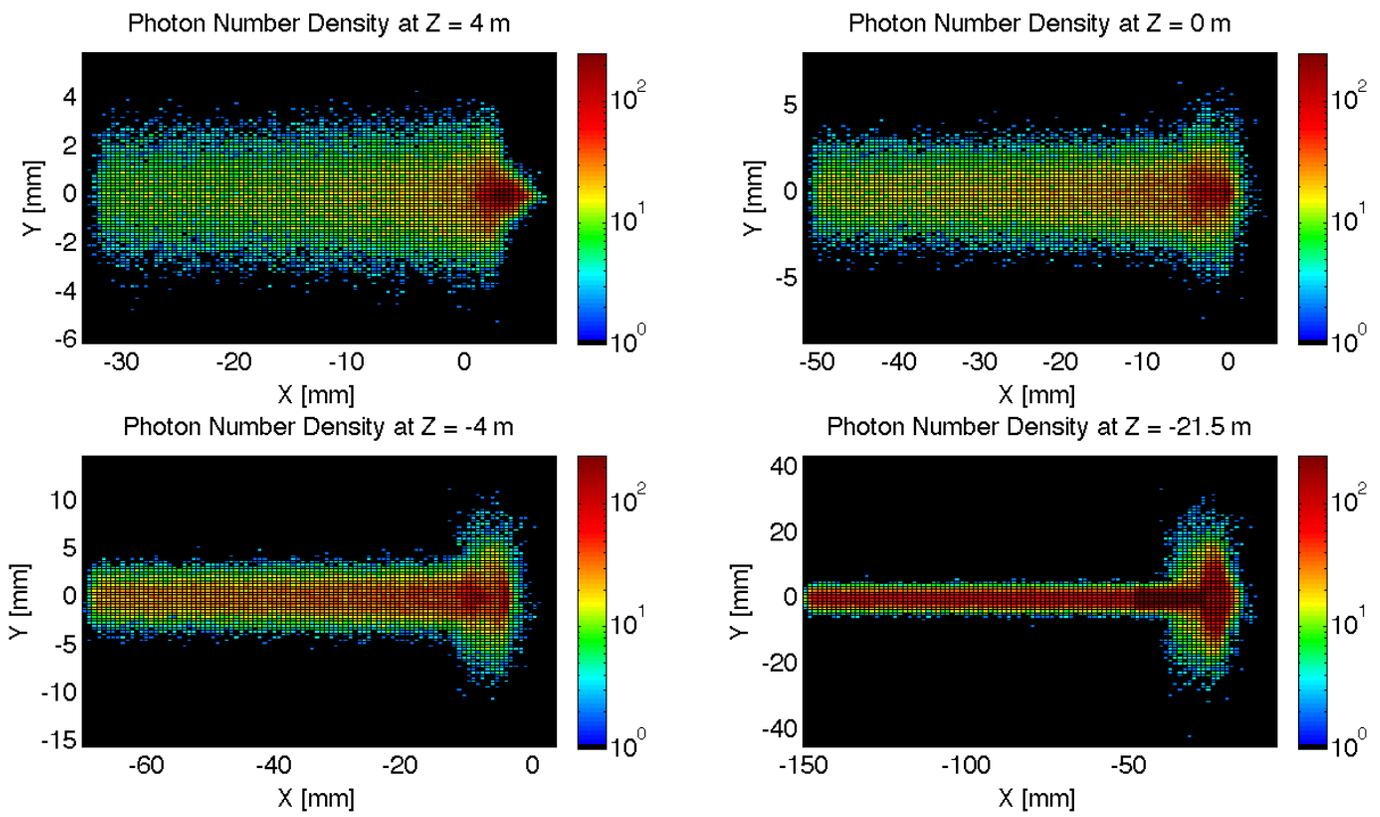
Figure 8.39: High Acceptance: Number Density Growth in Z
