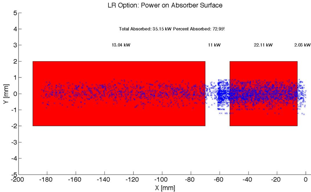
Figure 9.23: LR: Photon distribution on Absorber Surface
