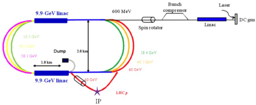
Figure 10.17: Layout of the injector assuming an injection at 600 MeV into the ERL.
