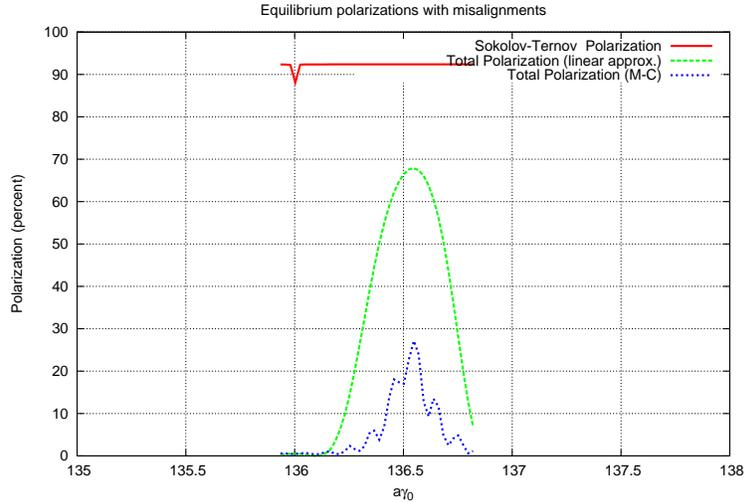
Figure 8.46: Estimated polarisation for the LHeC without spin rotators,  $Q_s = 0.1$ .
