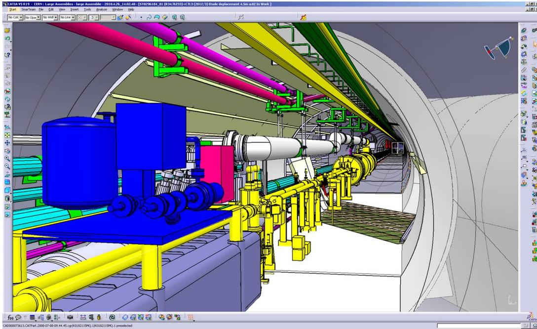
Figure 8.55: The cryogenic connection in point 3
