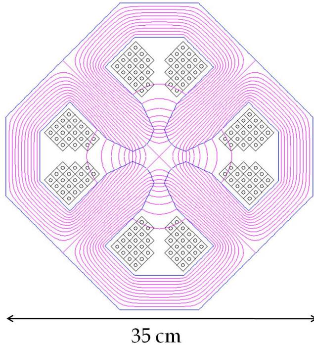
Figure 10.15: Quadrupoles for the recirculators of the LR option
