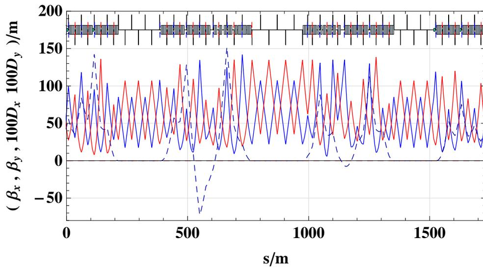
Figure 8.15: Bypass optics Point 1.
