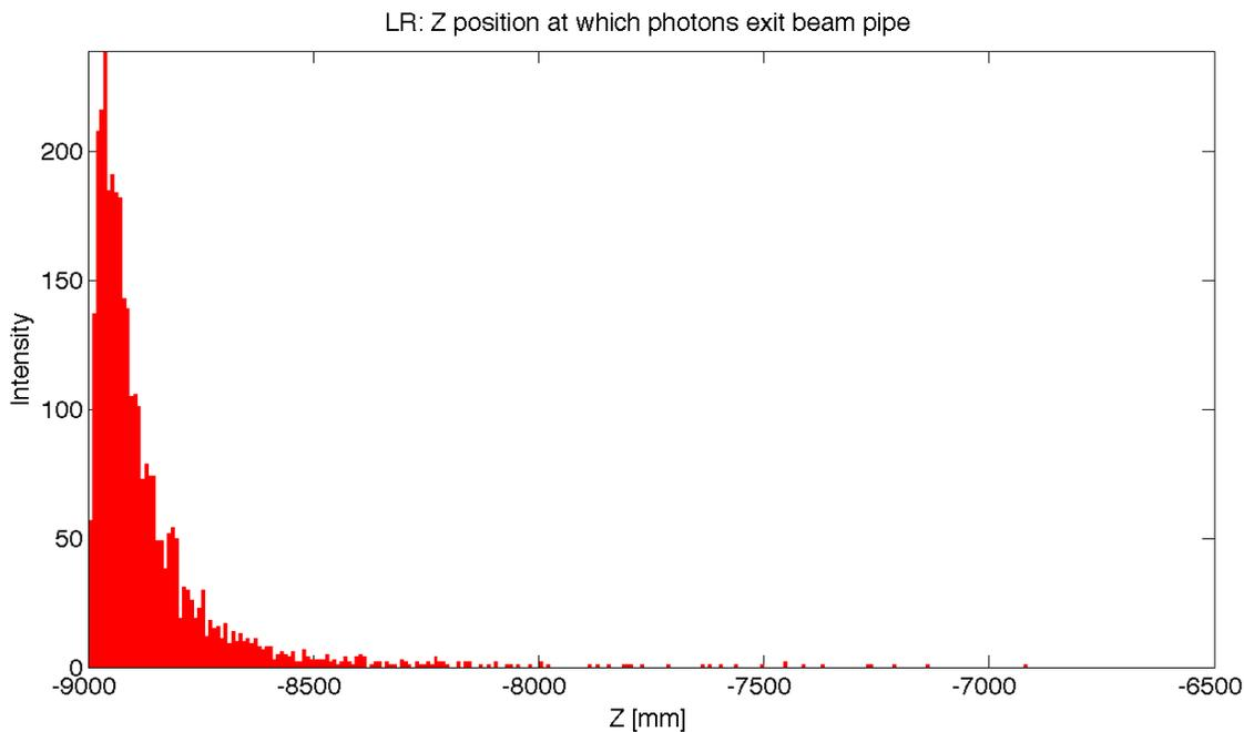
Figure 9.27: LR: Backscattered Photons Exiting the Beam Pipe
