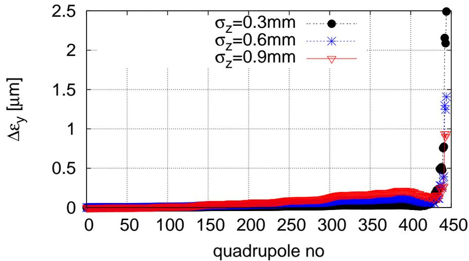
Figure 9.34: The single-bunch emittance growth along the LHeC linacs for a bunch with an initial offset of  $\Delta x = \sigma_x$ . The arcs have been represented by a simple transfer matrix.
