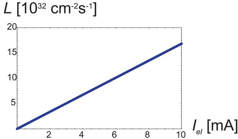
Figure 9.4: Linac-ring luminosity versus average electron beam current, according to (9.1).
