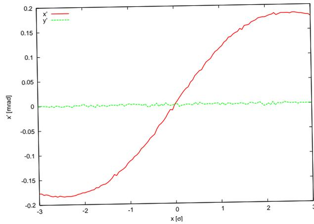
Figure 9.7: Simulated electron horizontal center-of-mass deflection angle as a function of the horizontal beam-beam offset.
