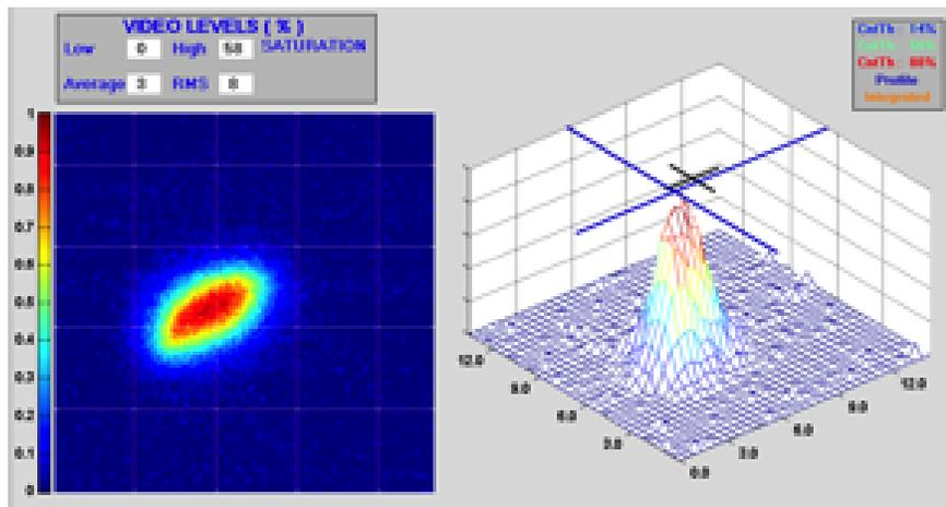
Figure 10.21: Electron beam profile at 500 MeV.
