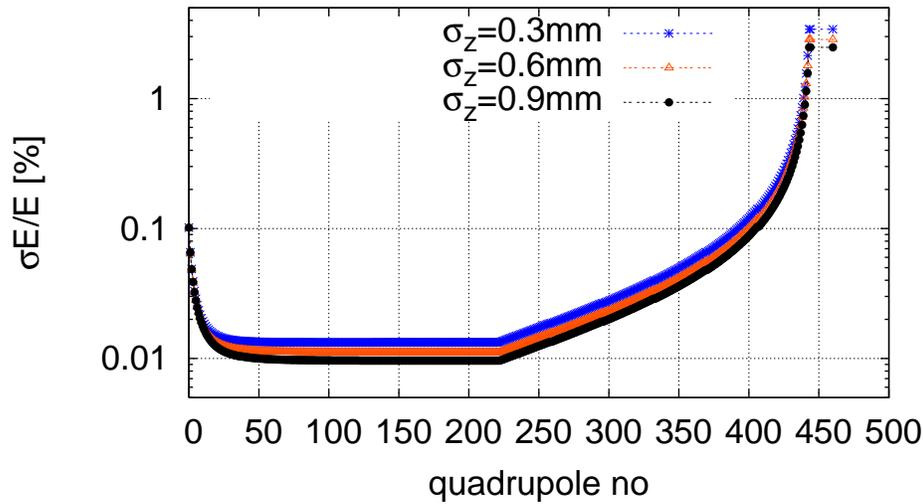
Figure 9.33: The RMS energy spread due to single bunch wakefields along the linacs. The bunch has been cut longitudinally at  $\pm 3\sigma_z$  and at  $\pm 3\sigma_E$  in the initial uncorrelated energy spread.
