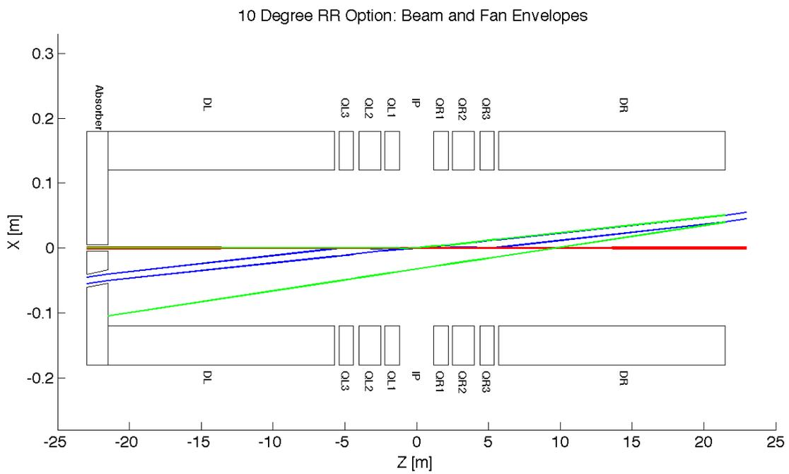
Figure 8.34: High Luminosity: Beam Envelopes in Z
