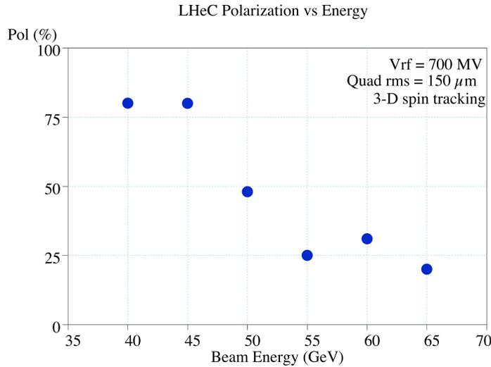
Figure 8.47: Equilibrium polarisation *vs* ring energy, full 3-D spin tracking results
