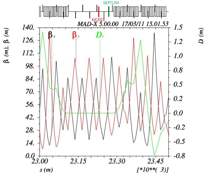
Figure 10.24: Injection optics is shown. The sequence starts ( $s=0$ ) at the beginning of the dispersion suppressor at the left side of IP2 and proceeds clockwise, while the electron beam rotates counterclockwise (from right to left in the figure). The injection kicker and septum are installed in the dispersion free region of the bypass at the right side of ATLAS.
