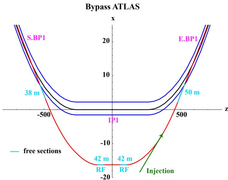
Figure 8.11: Bypass using the survey gallery in point 1. The LHC proton ring is shown in black, the electron ring in red and the tunnel walls in blue. Dispersion free sections reserved for the installation of RF, wiggler(s), injection and other equipment are marked in light blue. The injection is marked in green and is located in the right arc of the bypass. Beginning and end of the bypass are marked with S.BP1 and E.BP1
