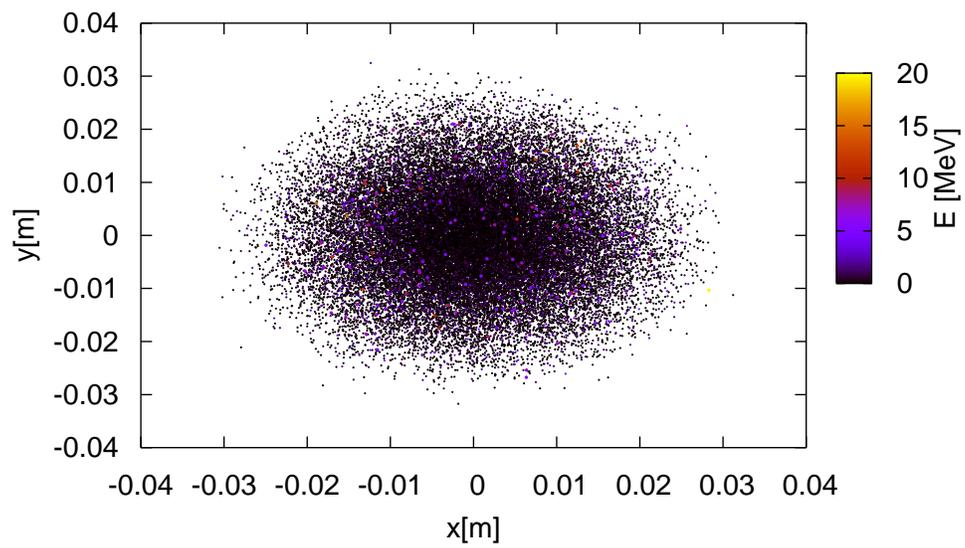
Figure 9.24: Beamstrahlung photons at the entrance of D1.
