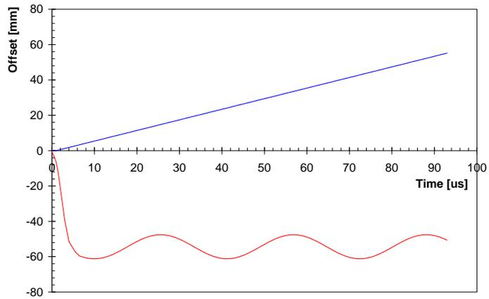
Figure 10.30: The strength of the vertical kicker oscillates in time by  $\pm 13\%$  around its nominal value. The deflection provided by the horizontal kicker increases almost linearly in time.
