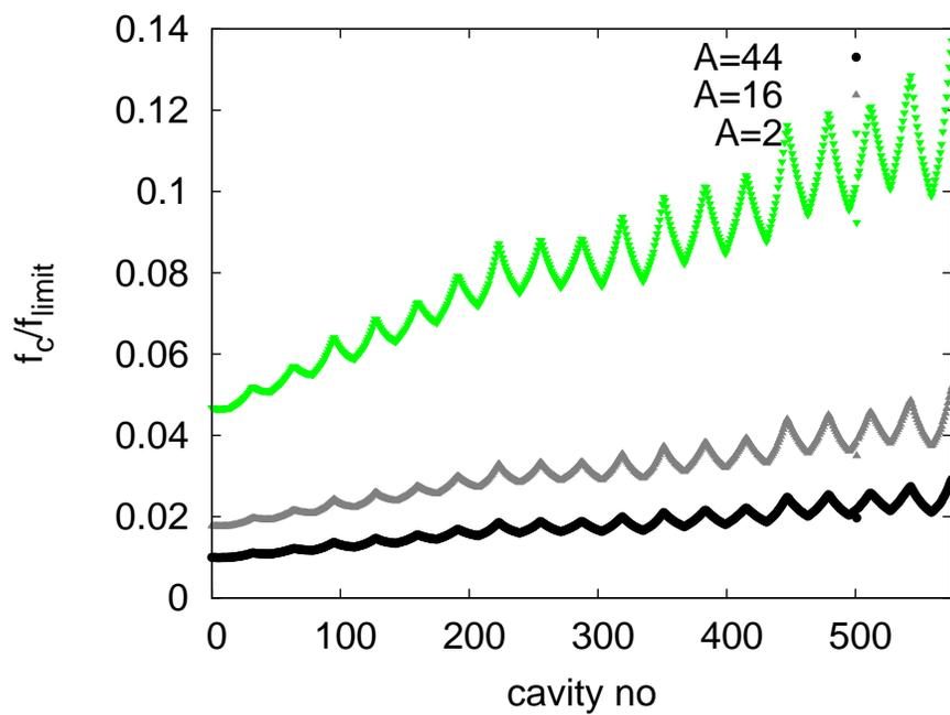
Figure 9.37: The oscillation frequency  $f_c$  of ions of different mass number  $A$  in the linacs using the average focusing strength of the bunches at different energy. The frequency is normalised to the limit frequency  $f_{limit}$  above which the ions would not be trapped any more.
