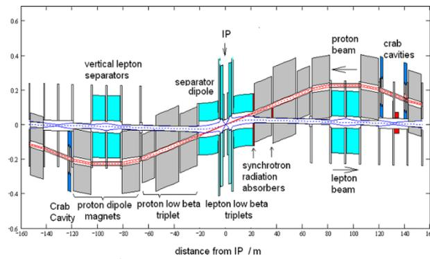
Figure 8.17: Schematic layout of the LHeC interaction region
