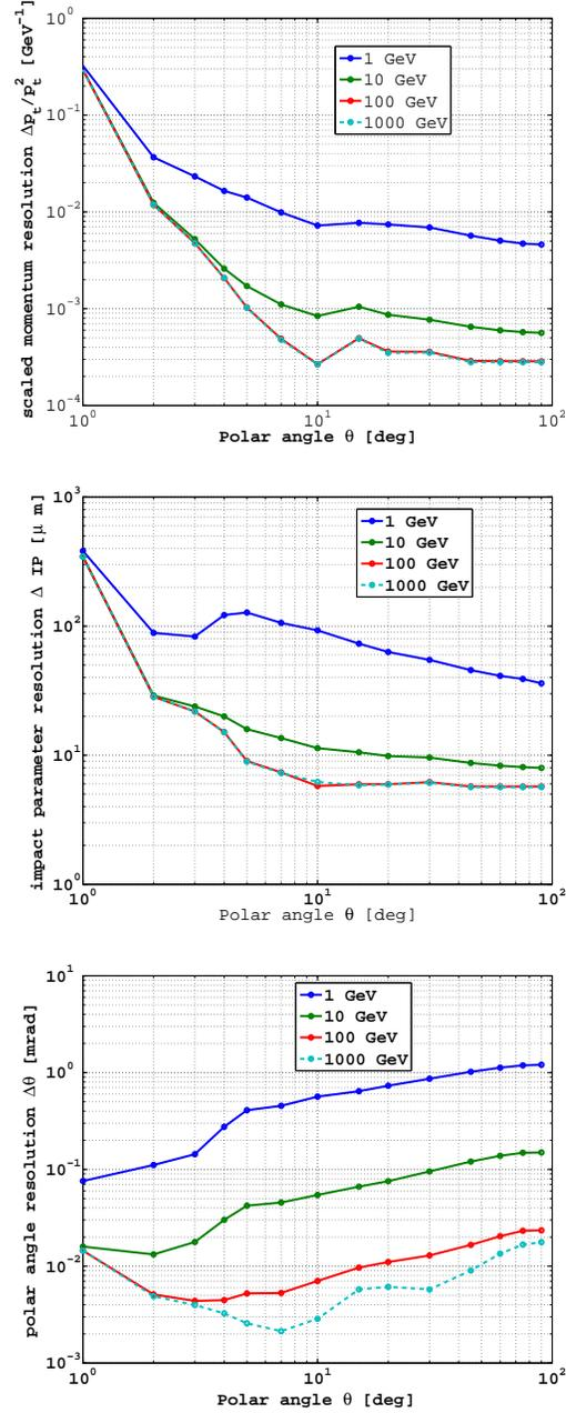
Figure 11.8: Transverse momentum (top), impact parameter (middle) and polar angle (bottom) measurement resolutions as function of the polar angle for the default detector design for four values of track transverse momentum.
