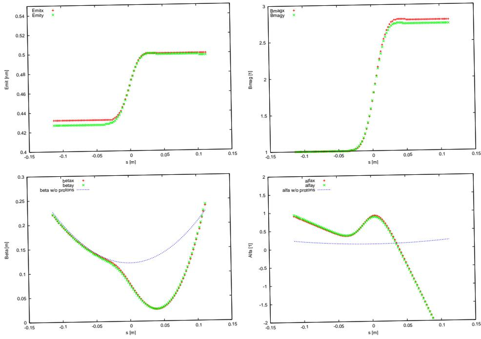
Figure 9.6: Simulated evolution of the electron beam emittance (top left), mismatch factor  $B_{\text{mag}}$  (top right) beta dfunction (bottom left) and alpha function (bottom right) during the collision with a proton bunch, as a function of distance from the IP.
