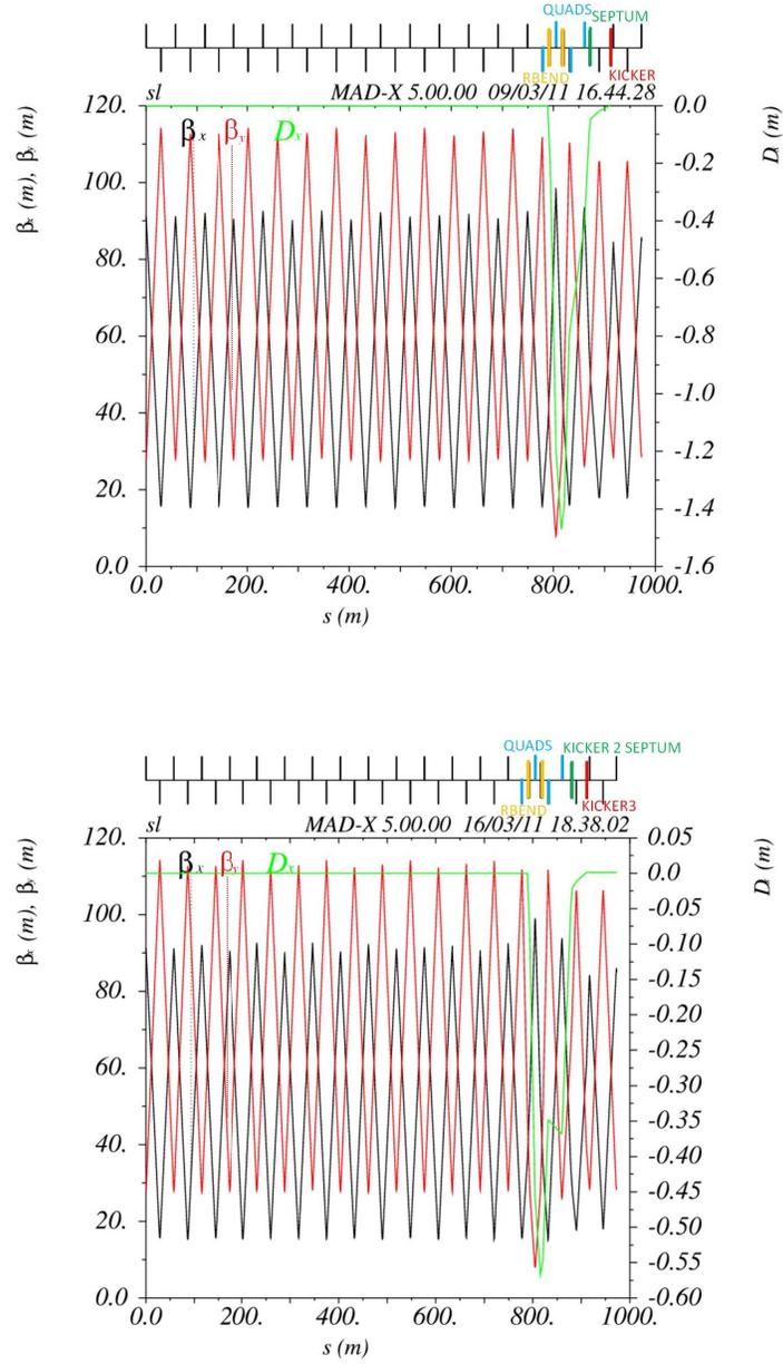
Figure 10.27: Transfer line optics for the injection onto orbit case (top) and mismatched injection case (bottom).
