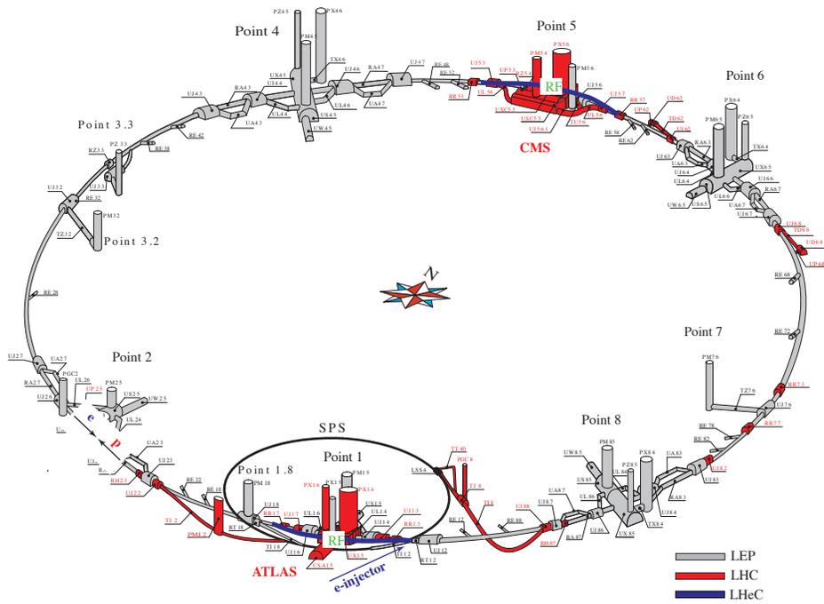
Figure 8.1: Schematic Layout of the LHeC: In grey the LEP tunnel now used for the LHC, in red the LHC extensions. The two LHeC bypasses are shown in blue. The RF is installed in the two bypasses. The bypass around point 1 hosts in addition the injection.
