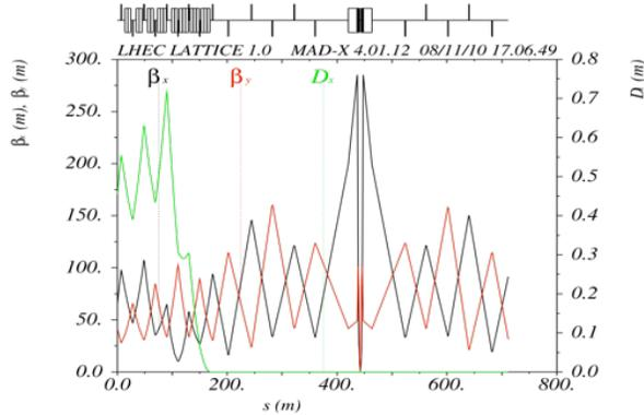
Figure 8.21: Electron optics for the LHeC interaction region. The plot corresponds to the 10 degree option where a triplet structure combined with a separation dipole has been chosen to separate the two beams.
