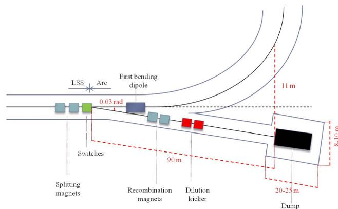
Figure 10.22: Scheme of the transfer line from end of long straight section of the linac and beam dump.
