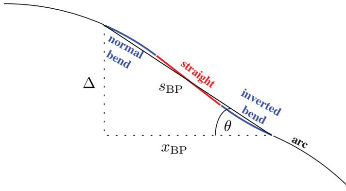
Figure 8.13: Outer bypass: a straight section is inserted to obtain the required separation. A larger separation could be achieved by inserting negative bends.
