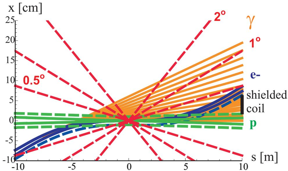
Figure 9.2: Linac-ring interaction-region layout. Shown are the beam envelopes of  $10\sigma$  (electrons) [solid blue] or  $11\sigma$  (protons) [solid green], the same envelopes with an additional constant margin of 10 mm [dashed], the synchrotron-radiation fan [orange], the approximate location of the magnet coil between incoming protons and outgoing electron beam [black], and a “1 degree” line.
