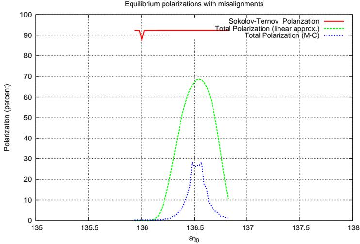
Figure 8.45: Estimated polarisation for the LHeC without spin rotators,  $Q_s = 0.06$ .
