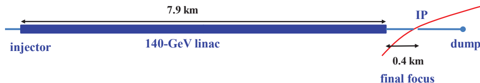
Figure 8.8: Pulsed single straight 140-GeV linac for highest energy ep collisions.
