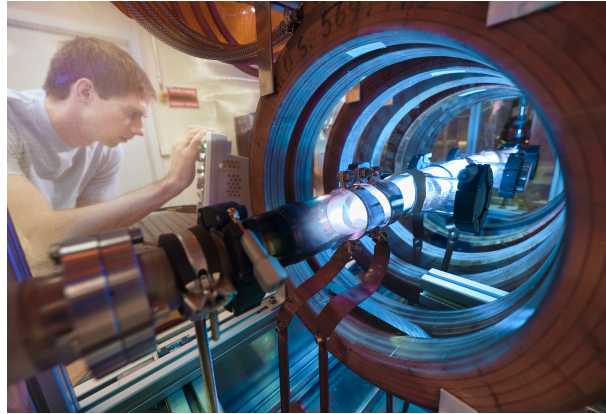
Fig. 3.11: 1 m prototype of a scalable Helicon plasma source. Image credit: CERN
