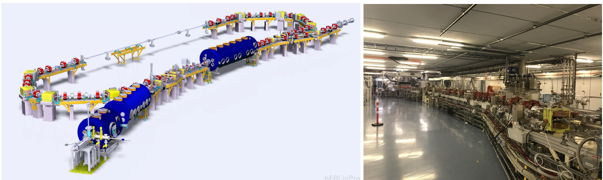
Fig. 5.2: Left: Structure of bERLinPRO, which is essentially complete apart from the 1.3 GHz linac module and the (upgraded) gun, the main hardware elements of the roadmap for bERLinPRO; Right: View from the dump position on the injector (at the back) and first racetrack part (June 2021).
