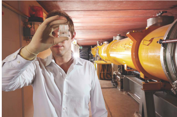
Fig. 4.3: A plasma cell is shown here in comparison to the super-conducting accelerator FLASH at DESY. Image credit: DESY, H. Mueller-Elsner
