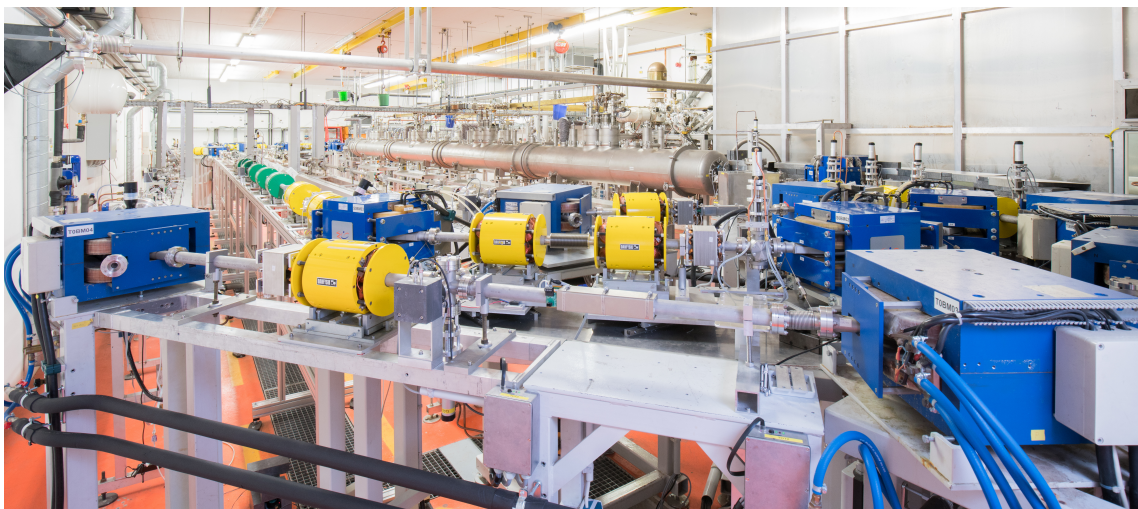
Figure 19. Photograph of the S-DALINAC with its three recirculation beam lines (by Jan-Christoph Hartung).
