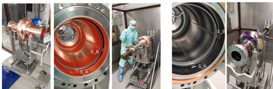
Figure 57. First Nb thin-film-coated 802 MHz cavity at CERN. The three leftmost figures show the copper cavity before coating including the clean-room assembly. The two rightmost figures show the cavity after the Nb coating [241].
