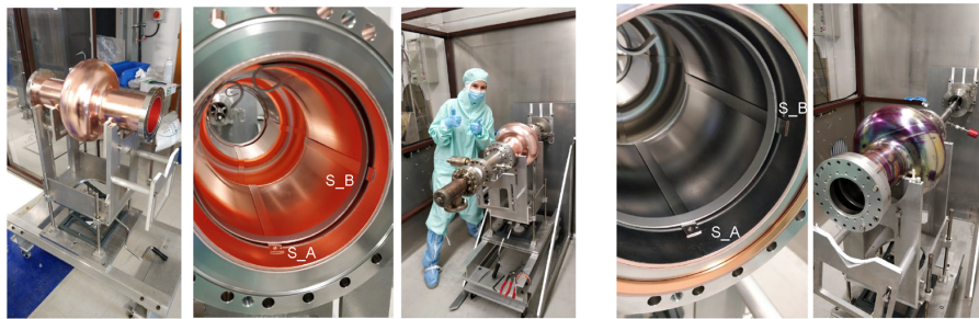
Figure 4.15. First Nb thin-film-coated 802 MHz cavity at CERN. The three leftmost figures show the copper cavity before coating including the clean-room assembly. The two rightmost figures show the cavity after the Nb coating [243].
