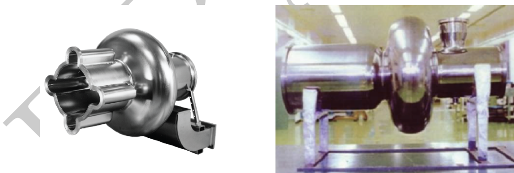
Figure 4.8.: The 500 MHz CESR cavity (left) [201], and 508 MHz KEKB cavity (right) [202]
