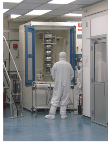
Figure 4.4.: JLab high-current ERL prototype cavities at 1.5 GHz (left) and 750 MHz during preparation (right) [195].
