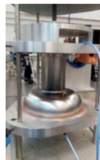
RF half cell/dumbbell measurements fixture
