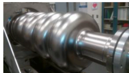
Five-cell cavity on tuning bench
