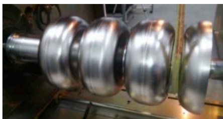
Five-cell cavity in EBW machine prepared for subsequent dumbbell and endgroup welding with both outside and inside welds in tilted position
