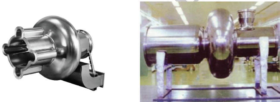
Figure 4.8.: The 500 MHz CESR cavity (left) [200], and 508 MHz KEKB cavity (right) [201]
