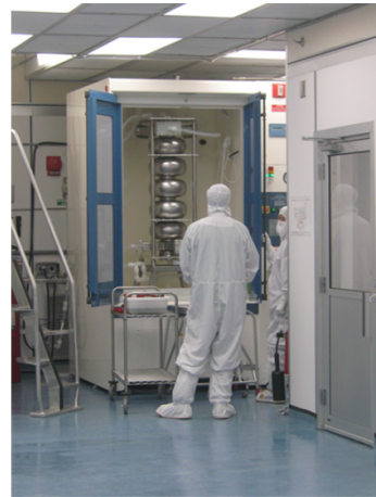
Figure 4.4.: JLab high-current ERL prototype cavities at 1.5 GHz (left) and 750 MHz during preparation (right) [194].
