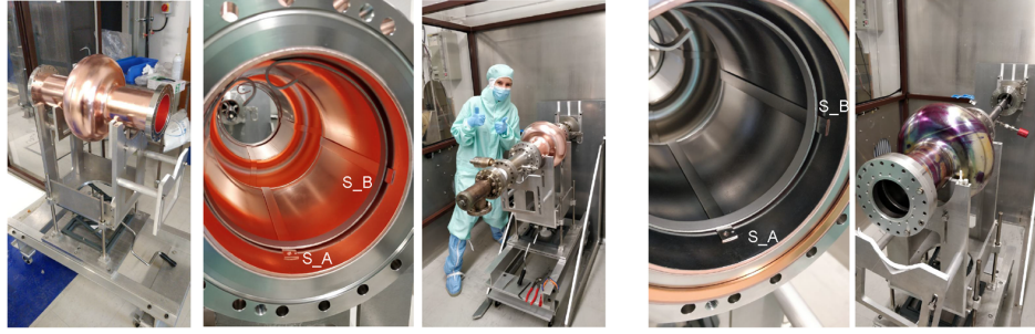
Figure 4.15.: First Nb thin film coated 802 MHz cavity at CERN. The three leftmost figures show the copper cavity before coating including the clean-room assembly. The two rightmost figures show the cavity after the Nb coating [228]
