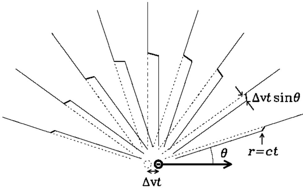
Figure 1: When an electron is accelerated, it carries its electric field along. The field further would only experience this drag at a slightly later time because signal cannot travel faster than light.
