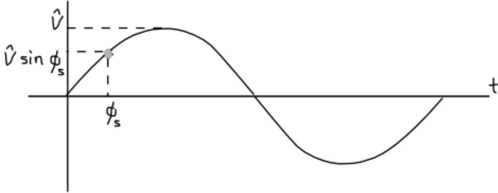
Figure 12: The energy gained by an electron in a cavity depends on the phase at which it enters the oscillating field.
