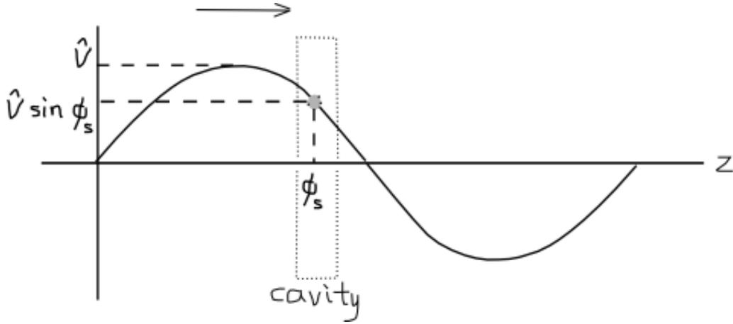
Figure 13: A “travelling” wave round the ring. This really exists only in the cavity, indicated by the dotted box.
