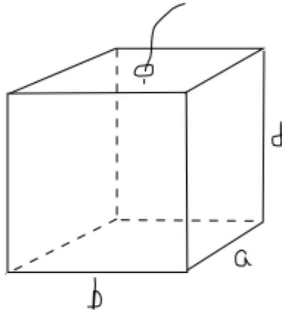
Figure 9: Current oscillating at the tip of the wire induces oscillating electric field in the metal box.
