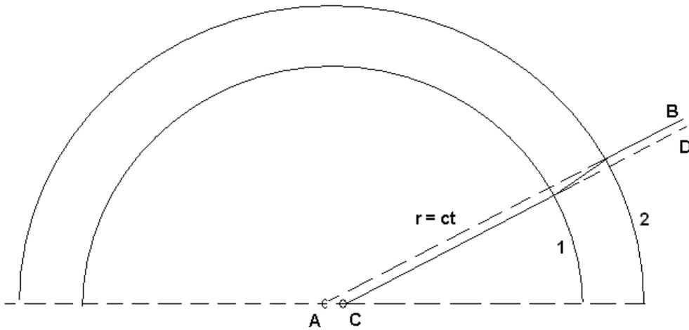
Figure 2: The effect of accelerating the electron for a short time is to produce a kink in the field that travels outward at the speed of light.
