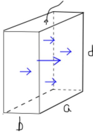
Figure 10: Choosing  $b$  to be the shortest side can result in a field that is parallel to side  $b$ .
