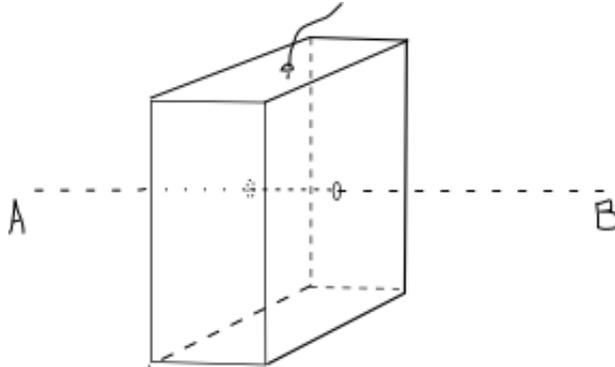
Figure 11: Making two tiny holes would not disturb the field very much.
