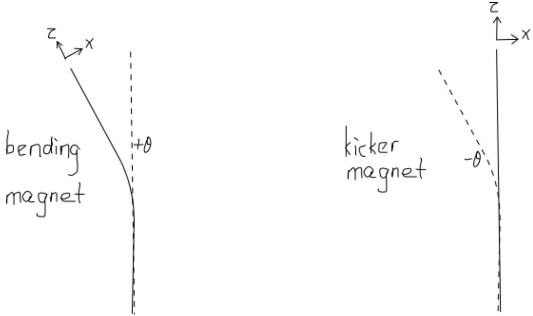
Figure 7: Bending magnet bends electrons to the design path. Kicker magnet kicks electron from the design path.
