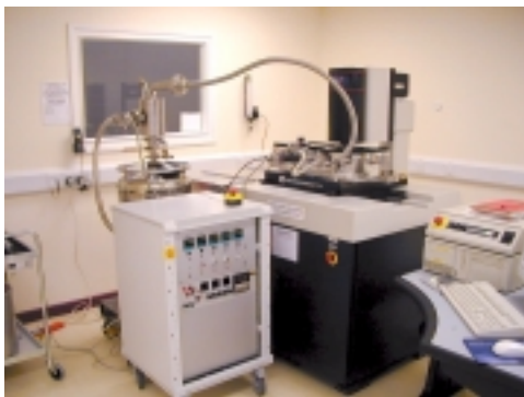
Figure 18: Survey cryostat with its cooling system mounted on the SmartScope CMM for the first measurements of temperature dependence of the shapes of stretched-silicon ladders.
