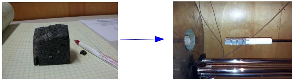
Crushed to reduce magnetisation for precise magnetometer measurement
