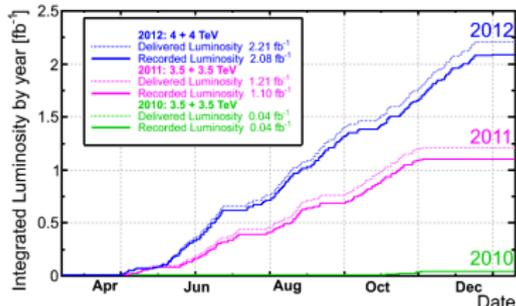
$L_{inst}^{Max} = 4 \times 10^{32} \text{cm}^{-2}\text{s}^{-1}$  (double the design value)
