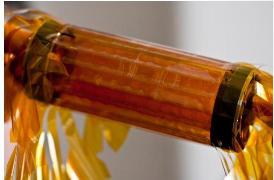
Vertex Prototype with 100 \mu\text{m} Glass
