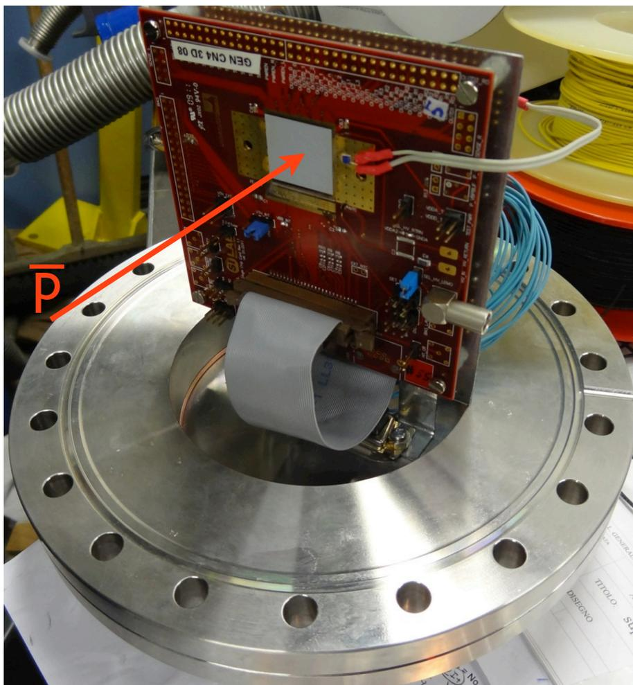
Strip sensors 50 and 80 μm pitch
