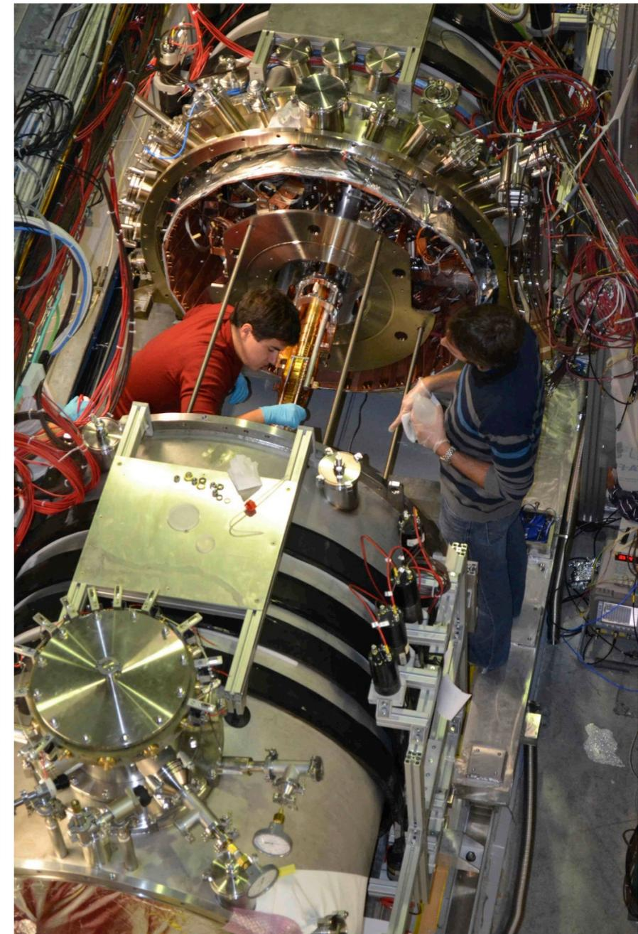
Assembly completed end of November 2012; immediate pump-down and cool-down (10 days) during which commissioning with antiprotons and positrons could take place
